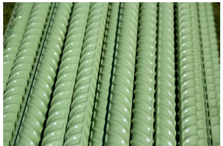
ECR resists corrosion and is the standard for Michigan bridge decks, but MDOT needed to quantify its performance. (Courtesy of iStockphoto.)
