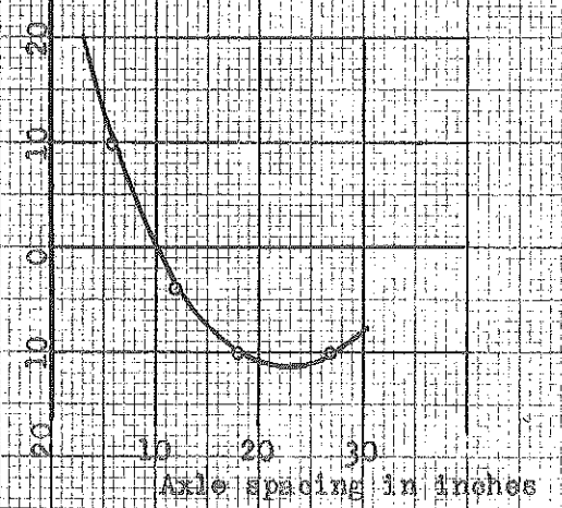
(C) Effect of 2nd load upon strain under first at edge of slab. ( 2 wheels per axle )
