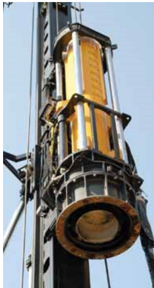
(a) Hydraulic Impact Hammer (Source: IMECO 2011)
