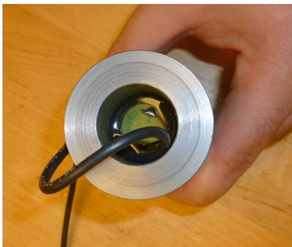
Figure 2-6 Geophone potted in push cone
