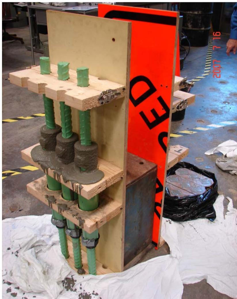
**Figure 3.7 Cast #11 NMB splices**
