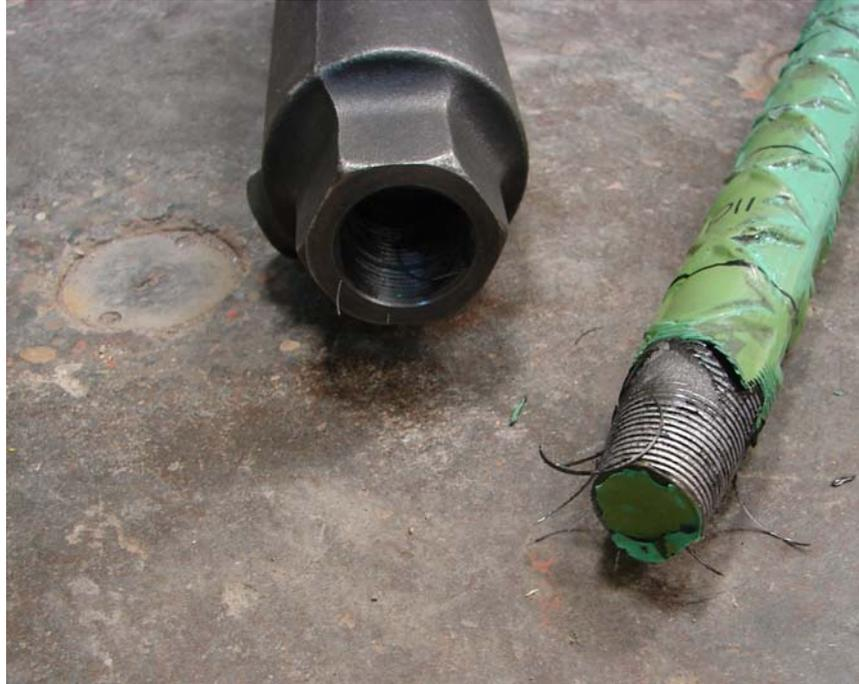
**Figure 4.24 Thread failure of specimen 11CI**
