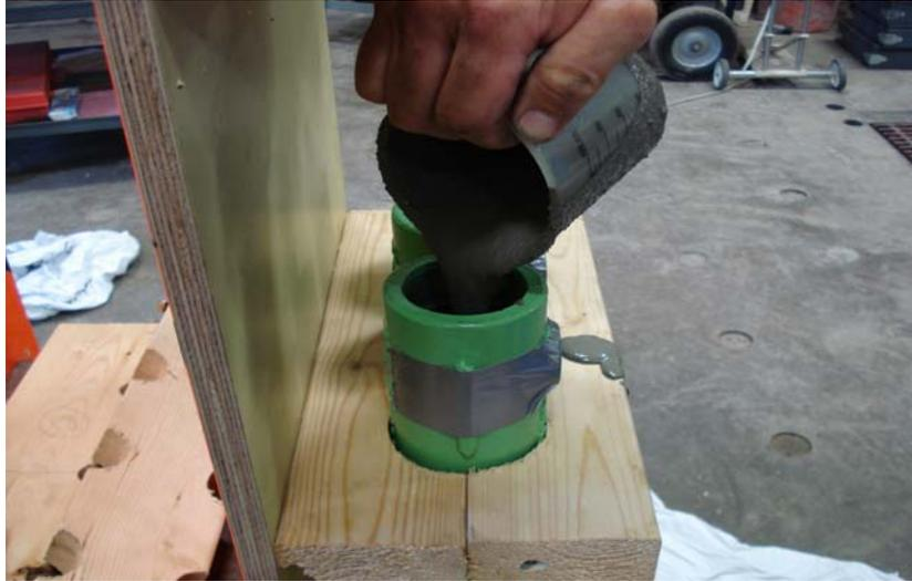
**Figure 3.4 Pouring grout in #11 NMB splices**
