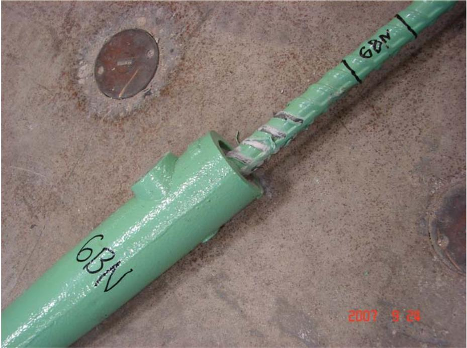
**Figure 5.21 Pull-out failure of specimen 6BN**
