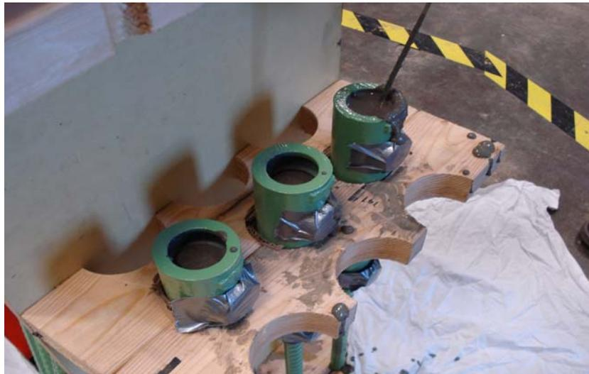
**Figure 3.5 Rodding grout in #6 NMB splices**
