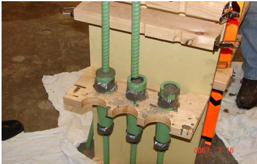
**Figure 3.6 Inserting #6 bars in NMB splices**
