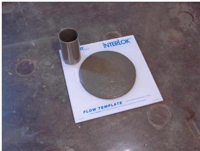
**Figure 3.3 Flow template for Nisso SS Mortar**
