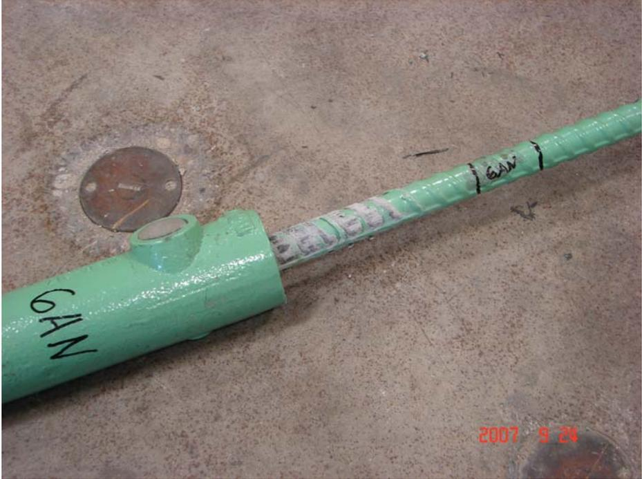
**Figure 5.20 Pull-out failure of specimen 6AN**
