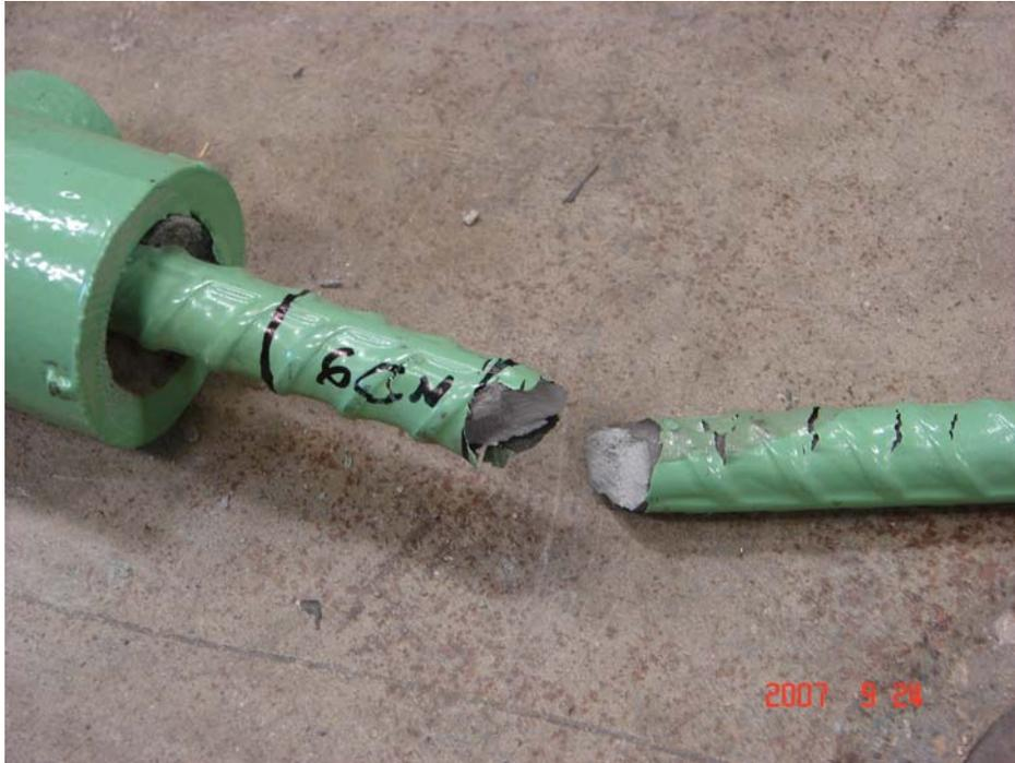
**Figure 5.22 Bar fracture of specimen 6CN**
