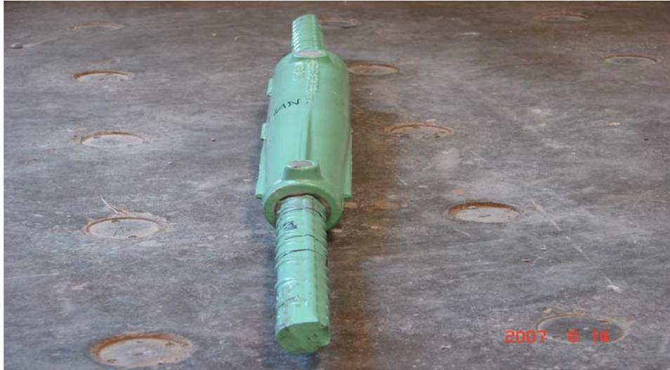
**Figure 5.1 Specimen 11AN after 65 kip compressive load**
