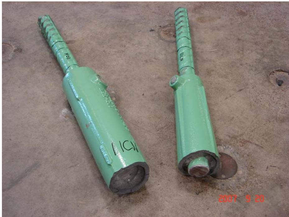
**Figure 5.25 Splice fracture of specimen 11CN**
