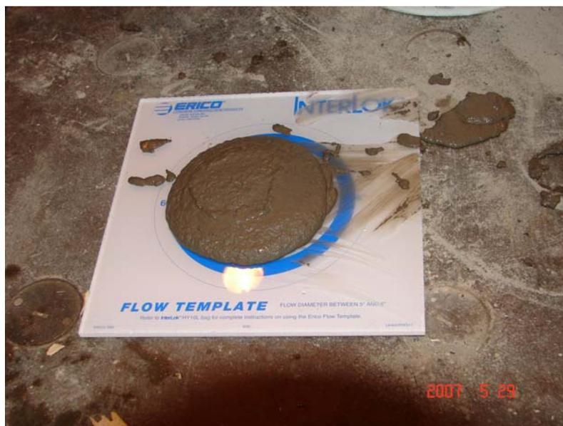
**Figure 3.2 Flow template for Erico HY10L Grout**
