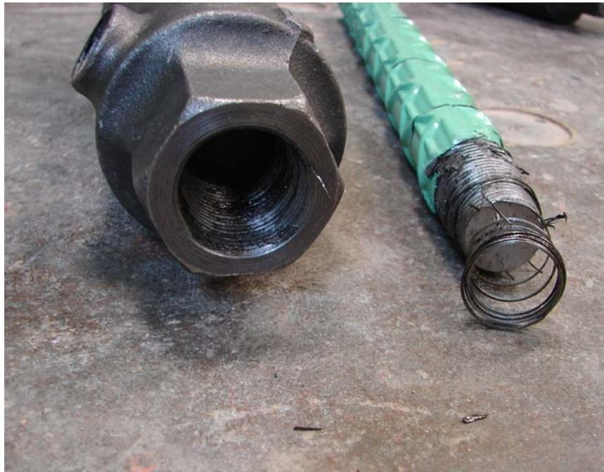
**Figure 4.23 Thread failure of specimen 11BI**
