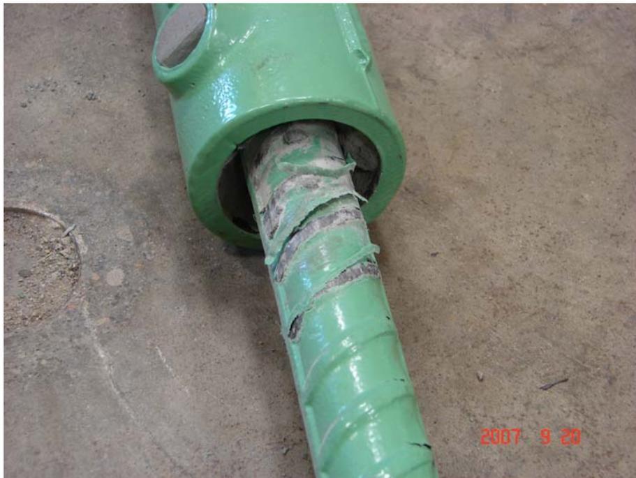
**Figure 5.23 Pull-out failure of specimen 11AN**
