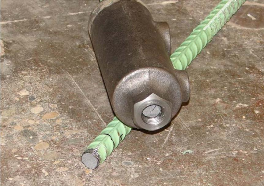
**Figure 4.20 Bar fracture of specimen 6CI**
