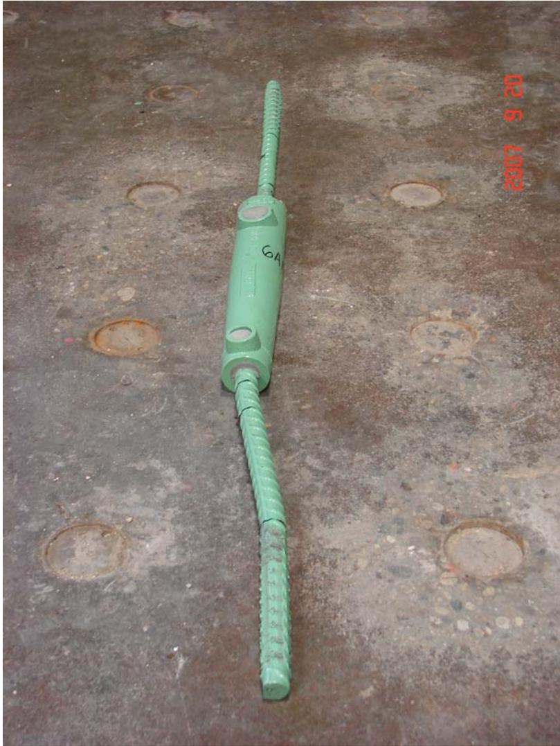
**Figure 5.13 Specimen 6AN after buckling**
