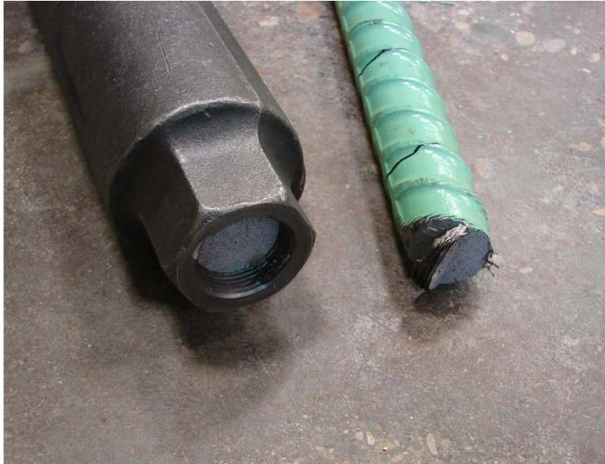
**Figure 4.22 Bar fracture at threads of specimen 11AI**
