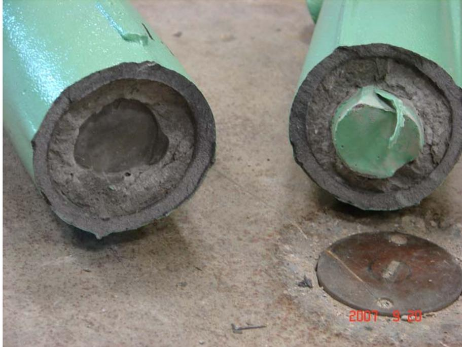
**Figure 5.24 Splice fracture of specimen 11BN**
