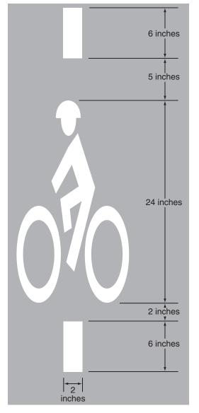
Figure 9C-7. Bicycle Detector Pavement Marking
