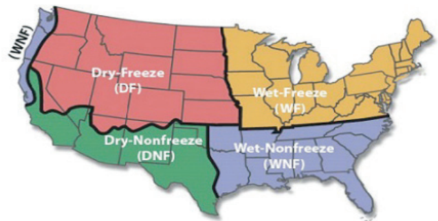
This map shows the four climate regions of the United States as designated by the FHWA for investigating long-term pavement performance.
