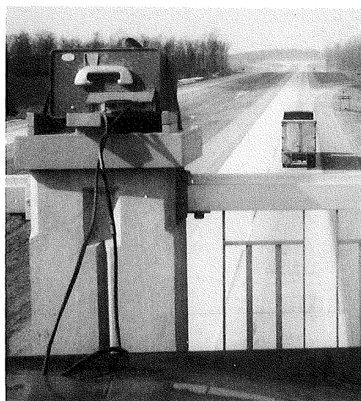
Figure 3. Hidden Detector Study of Vehicle Speeds on Freeway.
