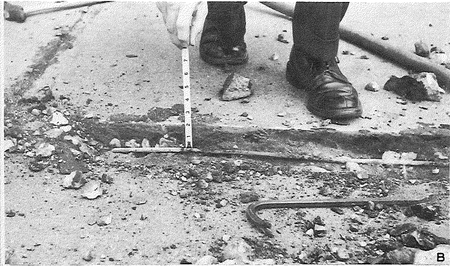
Figure 4. "Joint 3" where opening had occurred about 6 in. on the spalled side of the joint groove, is shown in an overall view (A). In the spalled area, reinforcement was embedded only 7/8- to 1 in. beneath the concrete surface (B). The reinforcing mat here was found to have been placed crosswise at the time of construction (C). A No. 4 gage wire was found to have broken within the slab, probably soon after construction (D, E), indicating that the pavement was opening at this point rather than at the joint. Muskegon Ave. at Ninth St.
