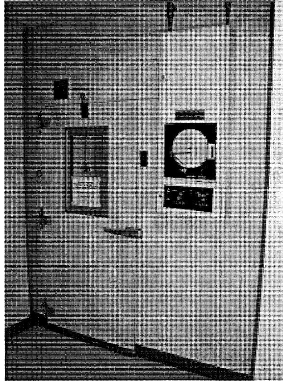
Photo 11-24. Exterior of thermal chamber
