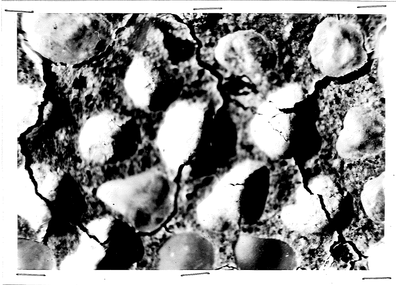
Figure 7 - Ottawa Sand Mortar - Treated with 30% Calcium Chloride 24 Hours
