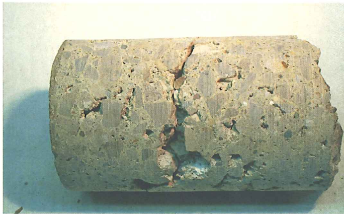
Figure 7. Honeycombing in core G2.
