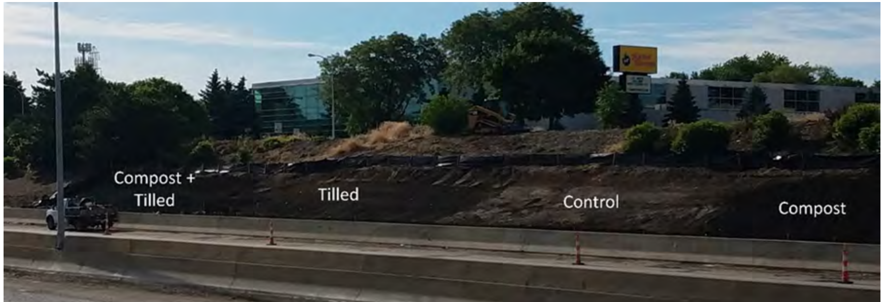
Figure 7. Plot layout of the four treatments (Control, Tilled Only, Compost only, and Compost and Tilled) within a block before plant installation.
