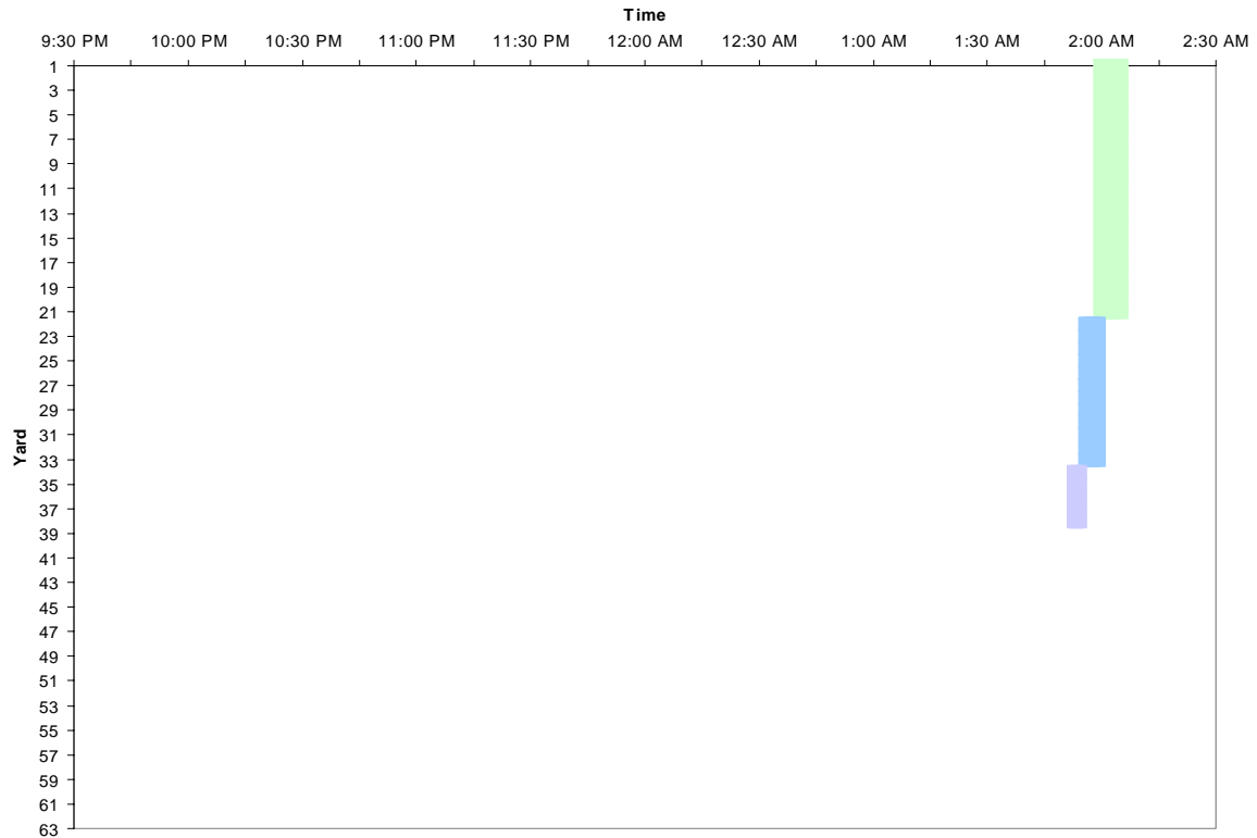
Figure 5-13. S06 of 82194, South section curing compound application time sequence
