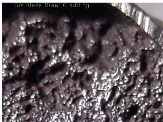
Figure 5. Magnified cross section (20x) of #6 size SCR showing pitting corrosion of the carbon steel. Note the stainless cladding in the upper right corner of the picture is unaffected (saw marks are visible).
