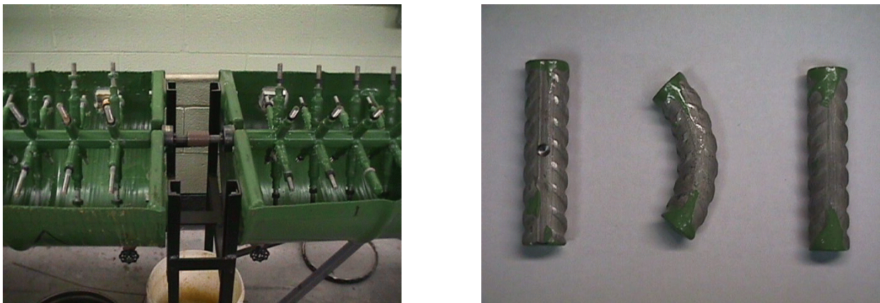
Figure 4. Corrosion test equipment and sample configuration for stainless-clad reinforcement testing.
