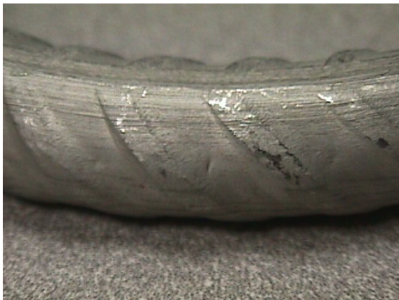
Figure 3. Cladding defect at outside of 3.75 in bend radius with #6 size SCR. Note the standard bend radius is 4.5 in for this size. The remaining #6 size samples and all #5 size samples passed bend testing.
