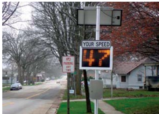
Figure 4: Actual Speed Feedback Sign Photo courtesy of FHWA
