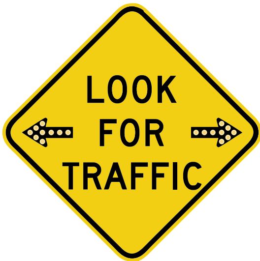
Figure 6: Minnesota’s “Look for Traffic” Sign – Both Arrows Flash when Traffic is Approaching
