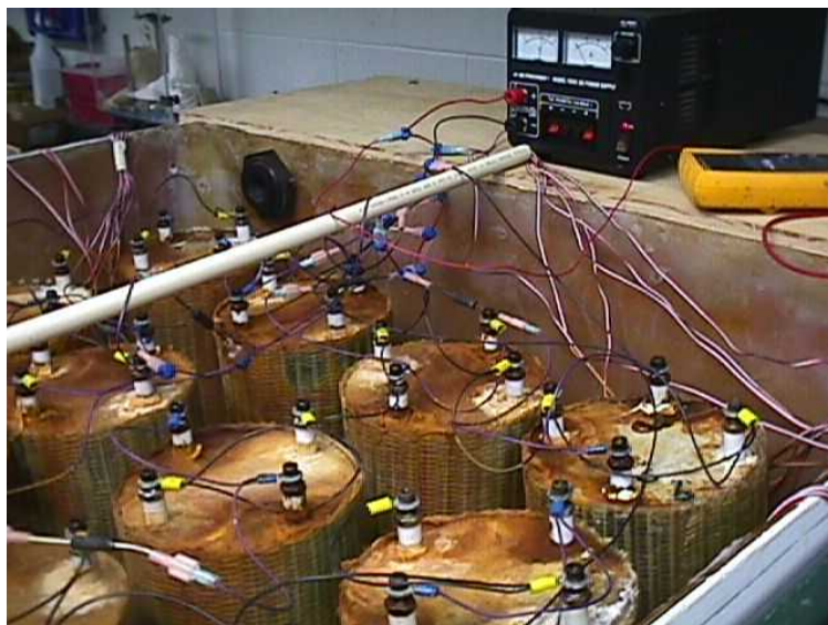
Fig. 2.12 Corrosion specimens in the tank
