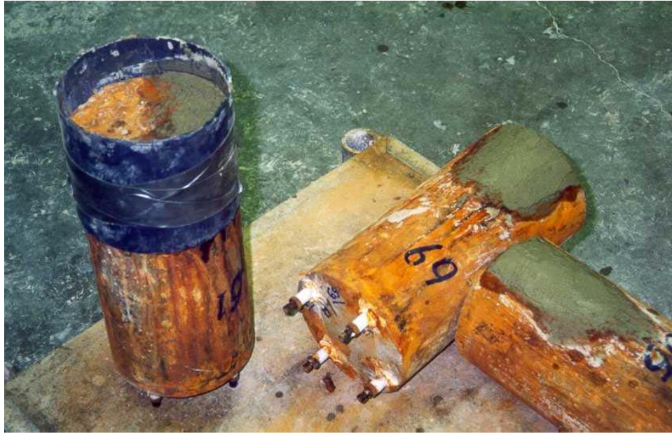
Fig. 2.10 Patching of the severely corroded specimens
