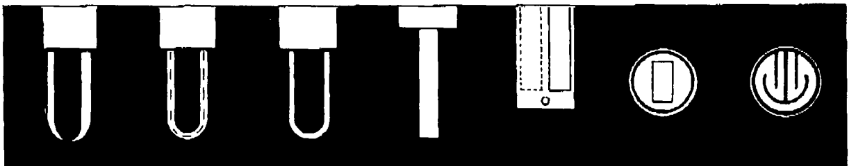
S4, S8 STRIP LOOP T4, T8 TUBE LOOP W40, W80 WIRE LOOP T10, T20, T50 CYLINDRICAL S4,* S8* ATMOSPHERIC S8* FLUSH END VIEW S10,* S20,* S40* FLUSH END VIEW
