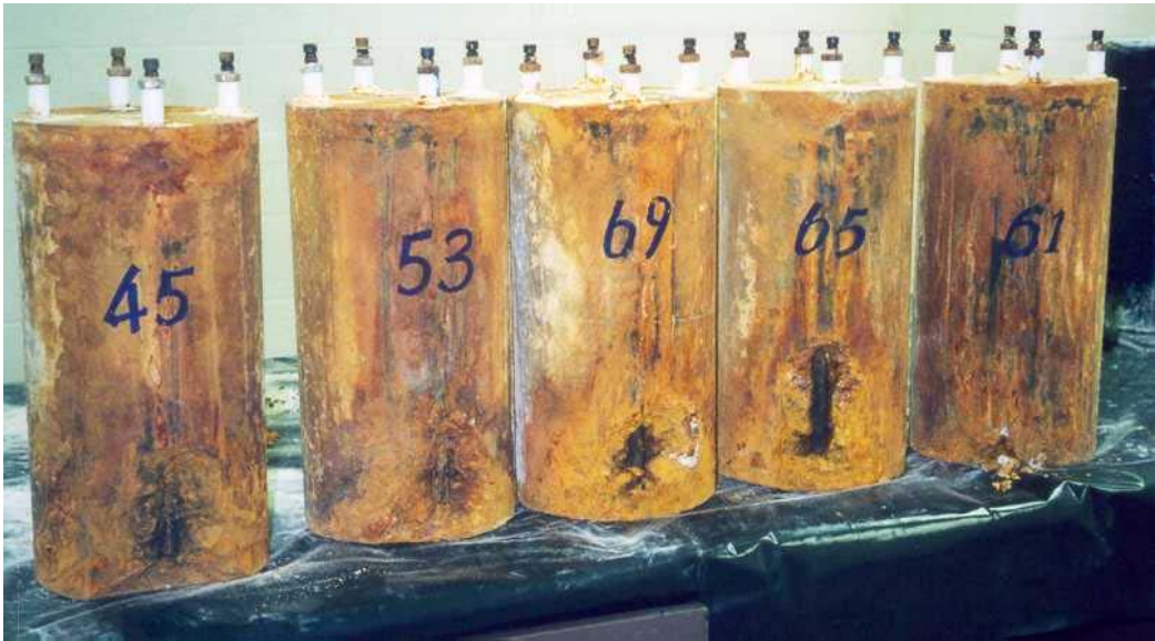
Fig. 2.9 Severely corroded specimens prior to patching
