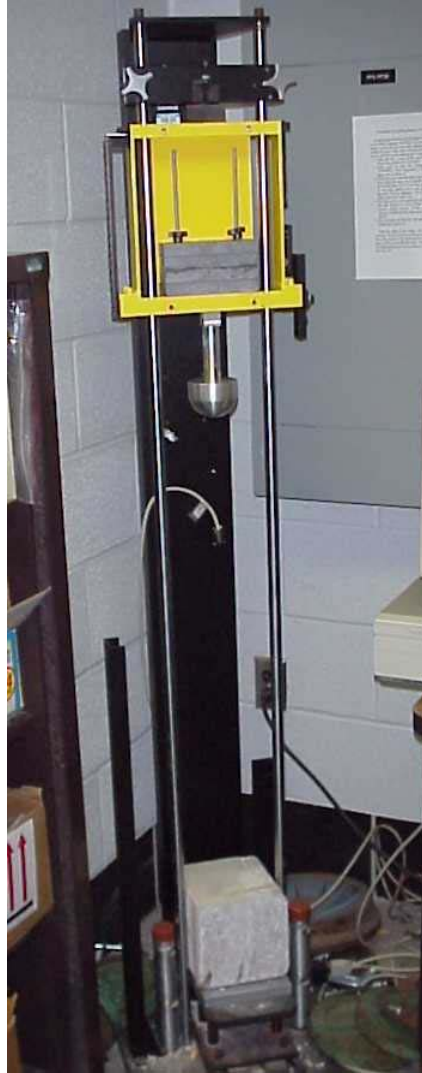
Fig. 2.17 Machine used for impact test of FRP panels
