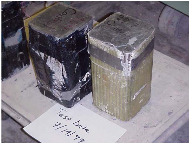
Fig. 3.36 Failure modes for square specimens under compression testing
