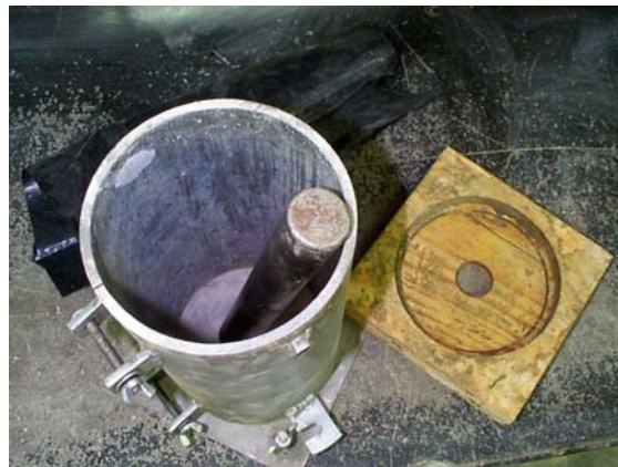
Fig. 2.2 Cylindrical mold used for freeze-thaw test specimens
