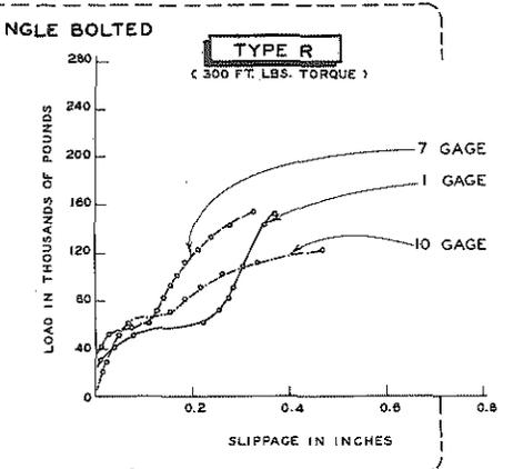
KEY: A, R, U, ETC. = TYPE DB = DOUBLE BOLTED 200, 300, ETC. = FT. LBS. BOLT TORQUE
