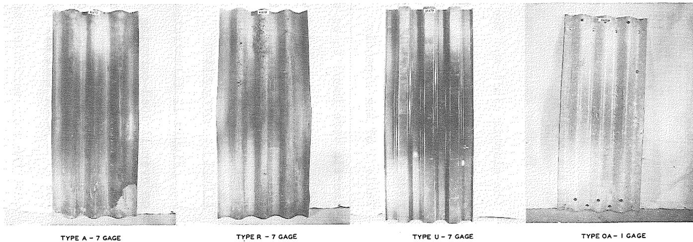
SPREADING OF SPECIMENS IN FAILURE - TEST I
