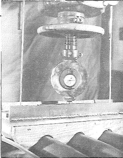
▲ FIGURE 10. METHOD OF DISTRIBUTING LOAD THROUGH BEAMS.
