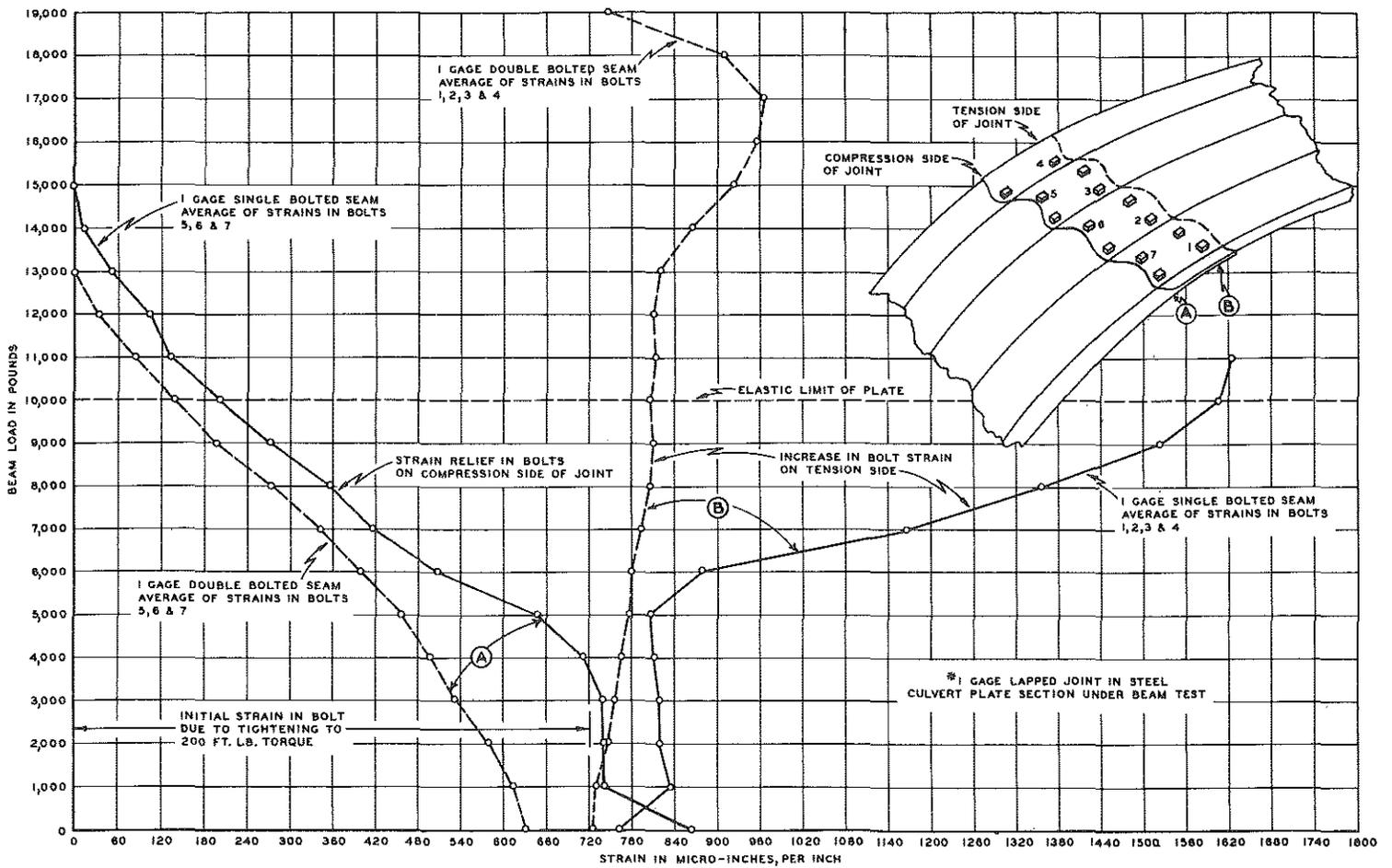
BOLT STRAINS IN DOUBLE AND SINGLE BOLTED LAPPED JOINT
