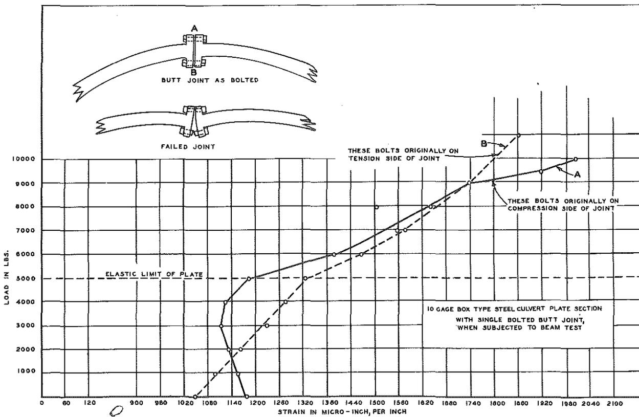
BOLT STRAINS IN BUTT JOINT
