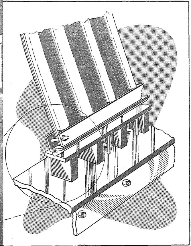
enough for 24-in. specimens. About half of the specimens in this test required a load greater than 75 tons and these were tested on the apparatus discussed above for Test 1. The upper head was lowered to allow for the difference in length between specimens 24 in. long and those 52-3/4 in. long. See Figure 4. Only the slippage at the joint between the two plates was measured for Test 2.
