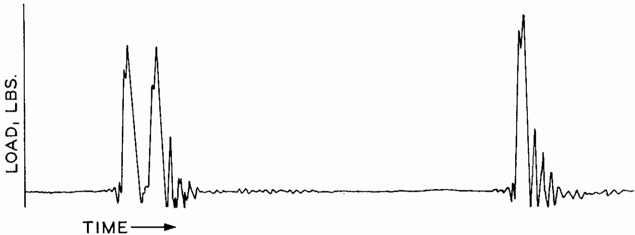
Figure 1. Typical wheel stopping forces obtained from static skid tester.
