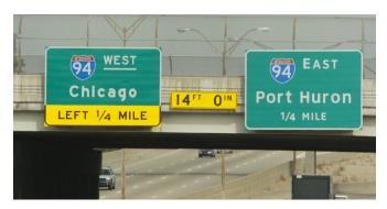
Signage changes to aid older drivers, reflected in the sign on the right, include lettering that decreases the nighttime halo effect, removal of underlining and enlargement of the first letter of the cardinal direction (east, west).
