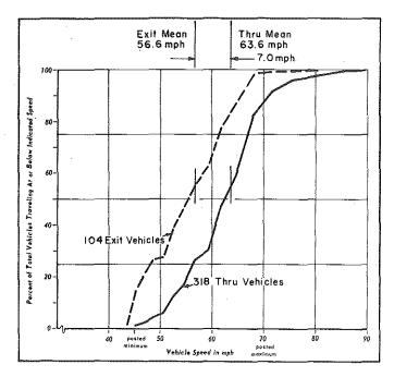
FIGURE 8. Thru and Exit Speeds 1-75 @ Dixie Highway (Enoscope Data)
