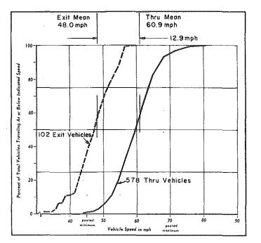
FIGURE 12. Thru and Exit Speeds US-27 @ Blanchard Rd. (Enoscope Data)
