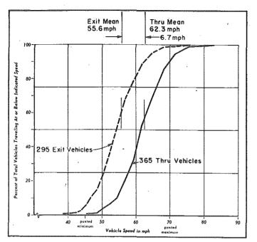
FIGURE 5. Thru and Exit Speeds US-127 @ M-36, (Enoscope Data)
