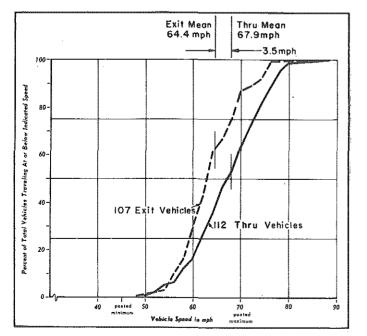
FIGURE 6. Thru and Exit Speeds US-127 @ M-36, (Electronic Data)
