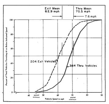
FIGURE 4. Thru and Exit Speeds I-96 @ US-127 (Enoscope Data)
