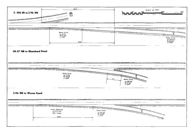
FIGURE 3. Horizontal Alignment of Taper Ramps
