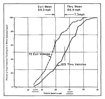
FIGURE 13. Thru and Exit Speeds US-27 @ Blanchard Rd. (Electonic Data)
