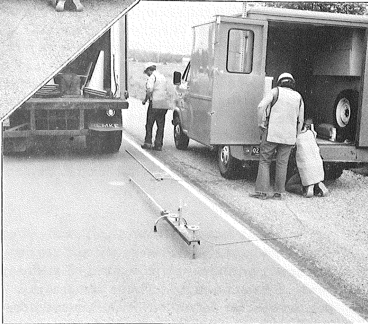
Recording deflections while the load truck is creeping forward.
