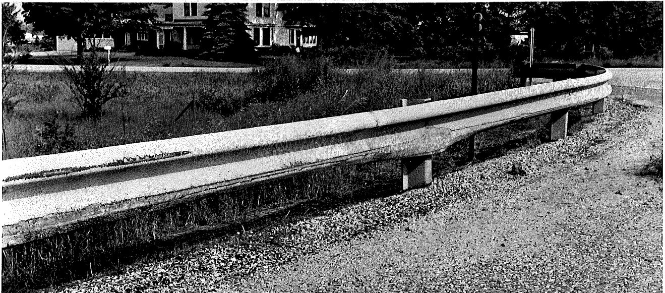
Figure 1. (top) Scraping damage on 50 ft of test guard rail at Knapp St. after four years of service. Gray granules overcoated the black binder.
