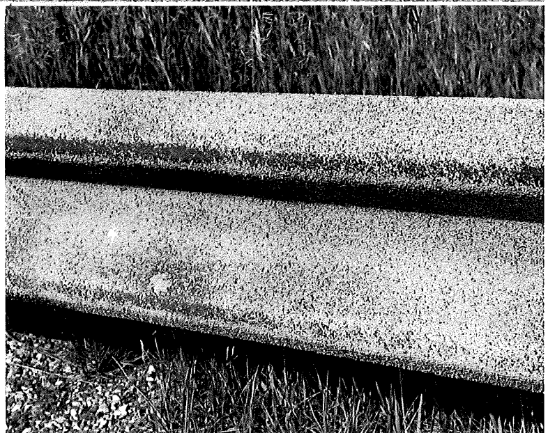
Figure 1. (top) Scraping damage on 50 ft of test guard rail at Knapp St. after four years of service. Gray granules overcoated the black binder.
