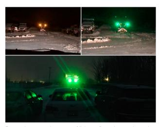
Researchers tested an array of light configurations to determine which setup maximizes visibility while minimizing glare.
