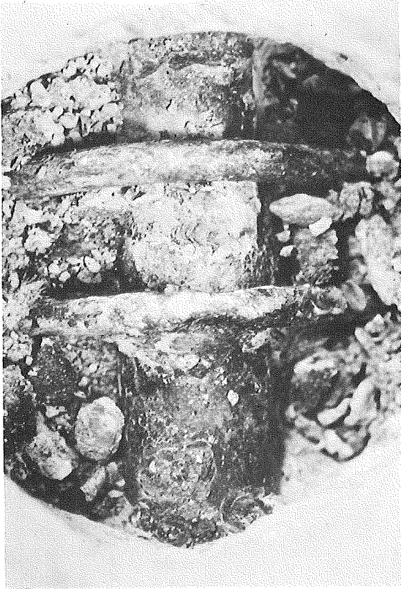
Figure 9 (above). Badly corroded standard hot-rolled steel dowels from one expansion joint assembly (Sta. 1127+30 WB), located first from pavement edge (left) and fifth from pavement edge (right).
