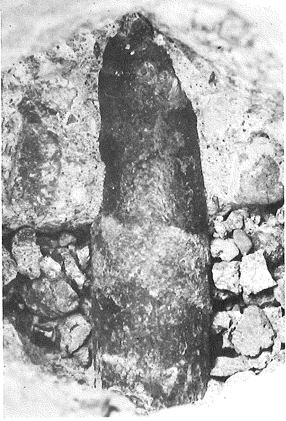
Figure 10 (below). Badly corroded standard hot-rolled steel dowels from one expansion assembly (Sta. 1130+00 WB), located first (left) and fifth (right) from pavement edge.
