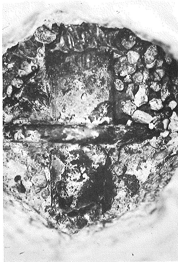
Figure 9 (above). Badly corroded standard hot-rolled steel dowels from one expansion joint assembly (Sta. 1127+30 WB), located first from pavement edge (left) and fifth from pavement edge (right).
