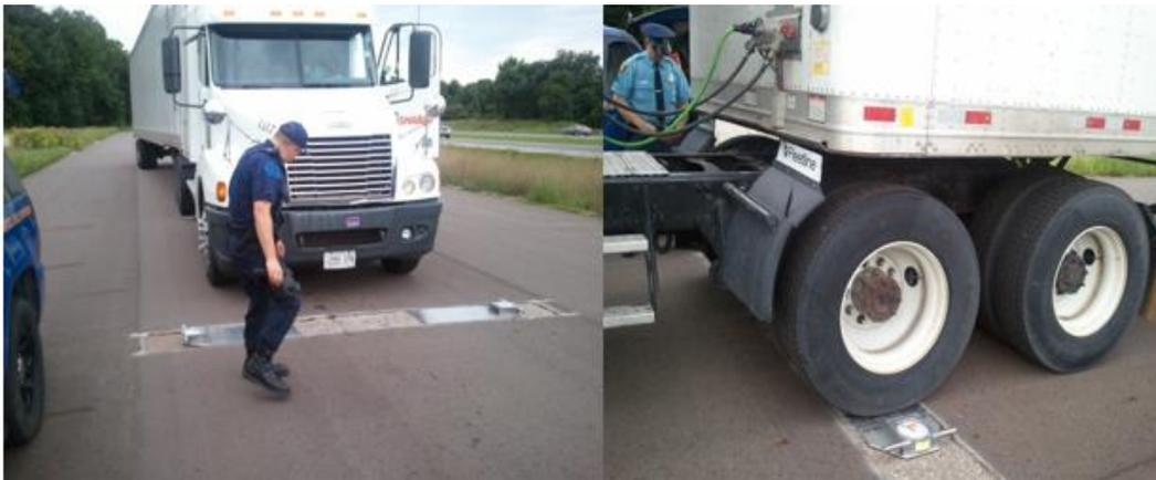
**Figure 2.3 Weighing a CMV using pavement cut-outs**
