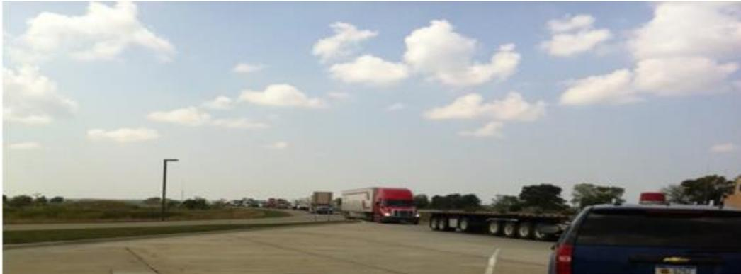
**Figure 4.13 A queue backup of trucks onto the mainline at a check-lane operation**
