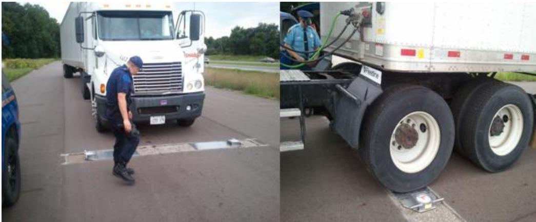
*(b) Weighing and inspecting the truck*
