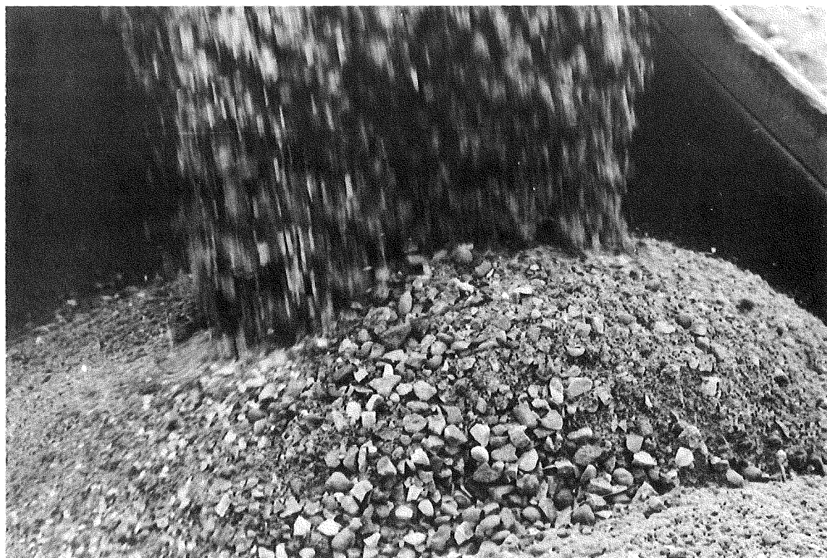
Figure 9. Segregation of rock salt as it falls into truck (salt falls to left).
