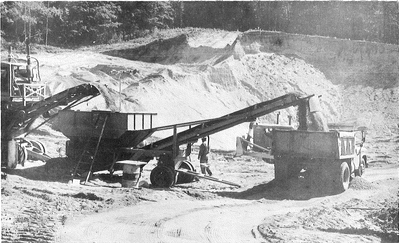
C. Belt feed to hopper. Drops to second belt for feeding to truck.
