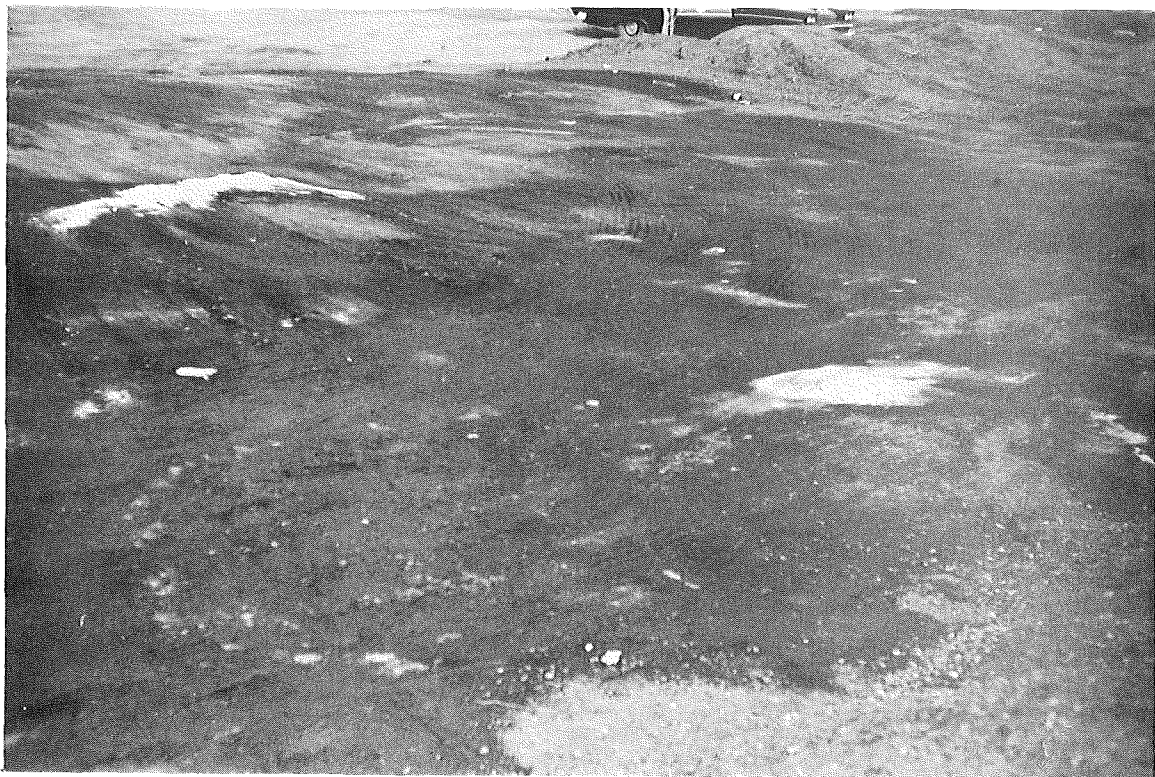
Figure 2. Appearance of stockpiles after surface addition of calcium chloride. Darker areas indicate recently dissolved chloride.
