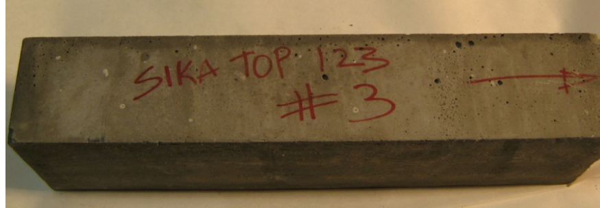
Figure F-13. Photograph of Sika Top 123 PLUS at the End of 300 Cycles of Freezing and Thawing
