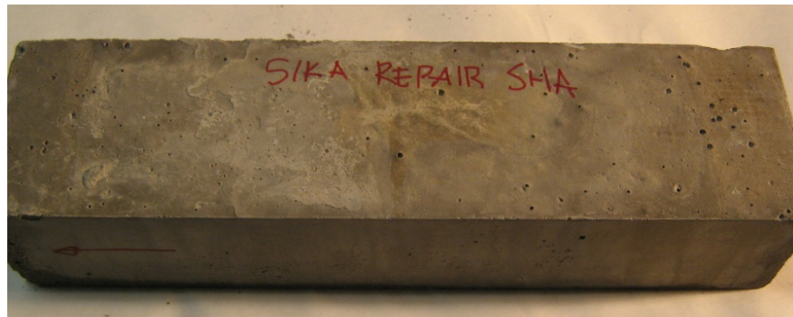
Figure F-14. Photograph of Sika Repair SHA at the End of 300 Cycles of Freezing and Thawing
