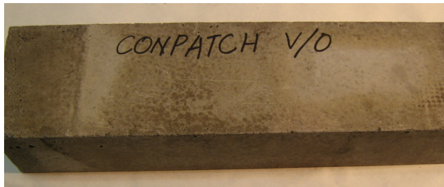
Figure F-15. Photograph of Conpatch VO at the End of 300 Cycles of Freezing and Thawing
