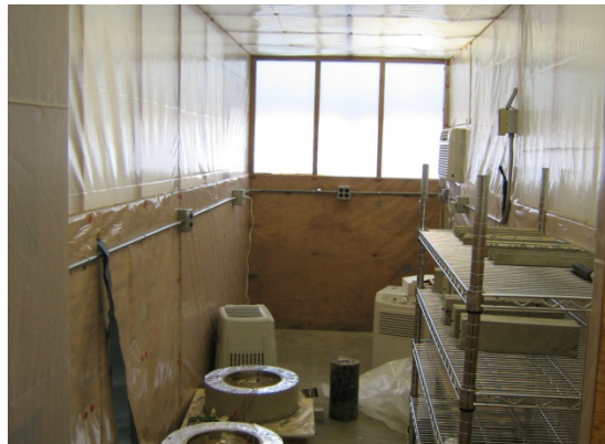
Figure 4-10. Environmental control chamber with ring specimen
