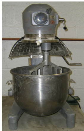
Figure 4-4. Hobart mixer used for mixing repair materials
