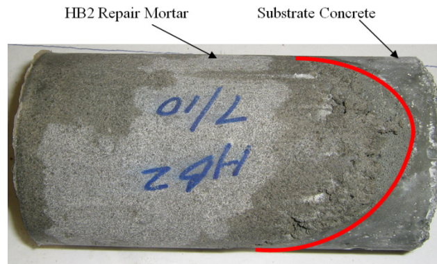
Figure 5-5. Voids in HB2 repair mortar specimen for slant shear bond strength test
