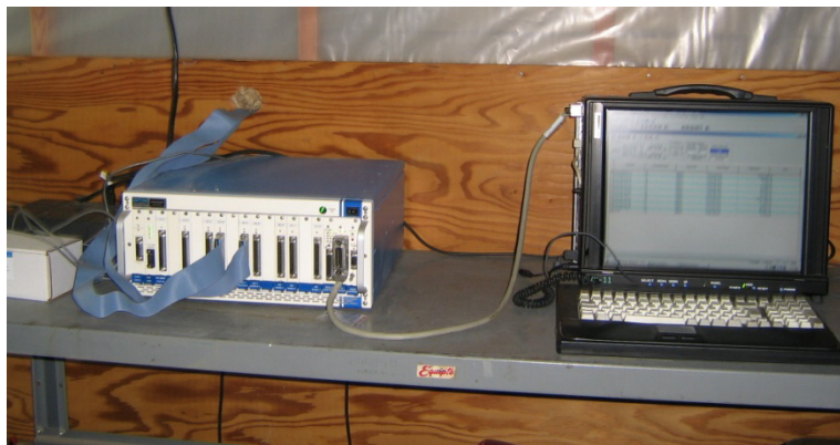
Figure 4-11. Data logger used for data collection from ring specimens
