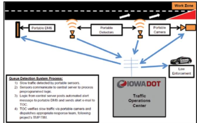
Figure 3: Queue Detection System. (Source: Iowa DOT)
