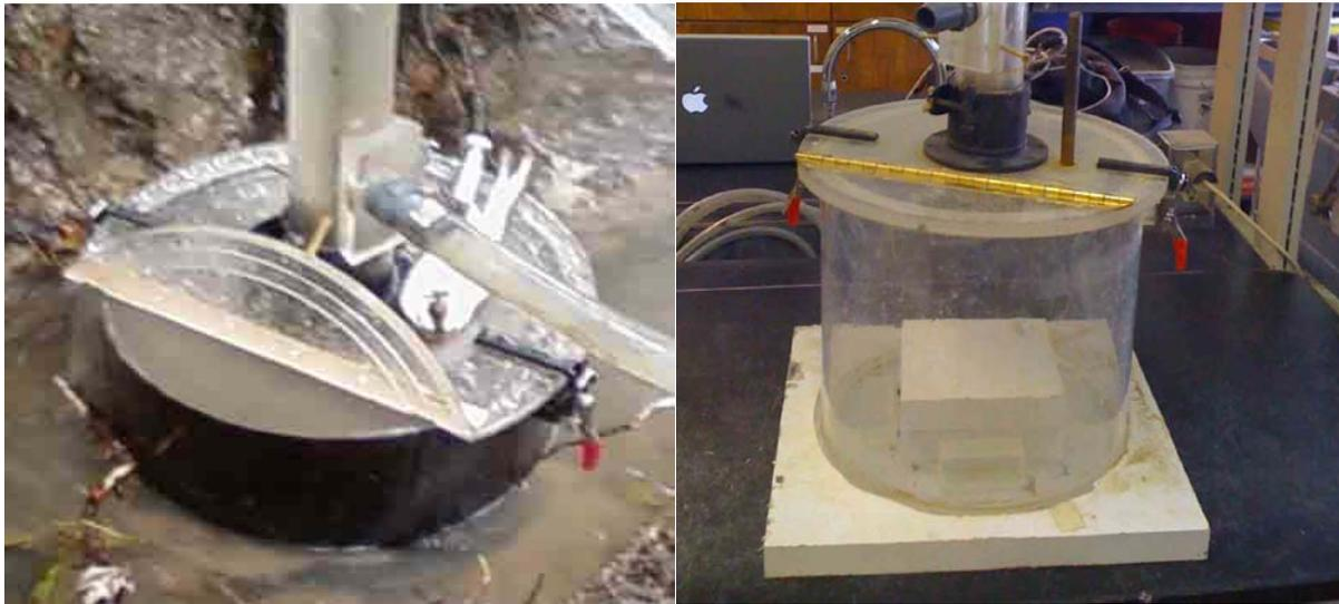
**Figures 6.3 (a)** Submergence tank and lid      **(b)** Lab tank and lid
