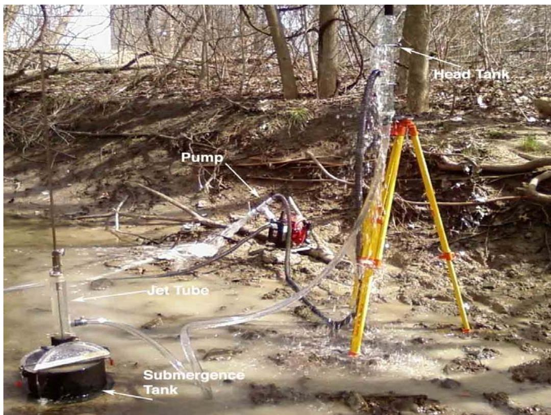
**Figure 6.8** JET apparatus in the field
