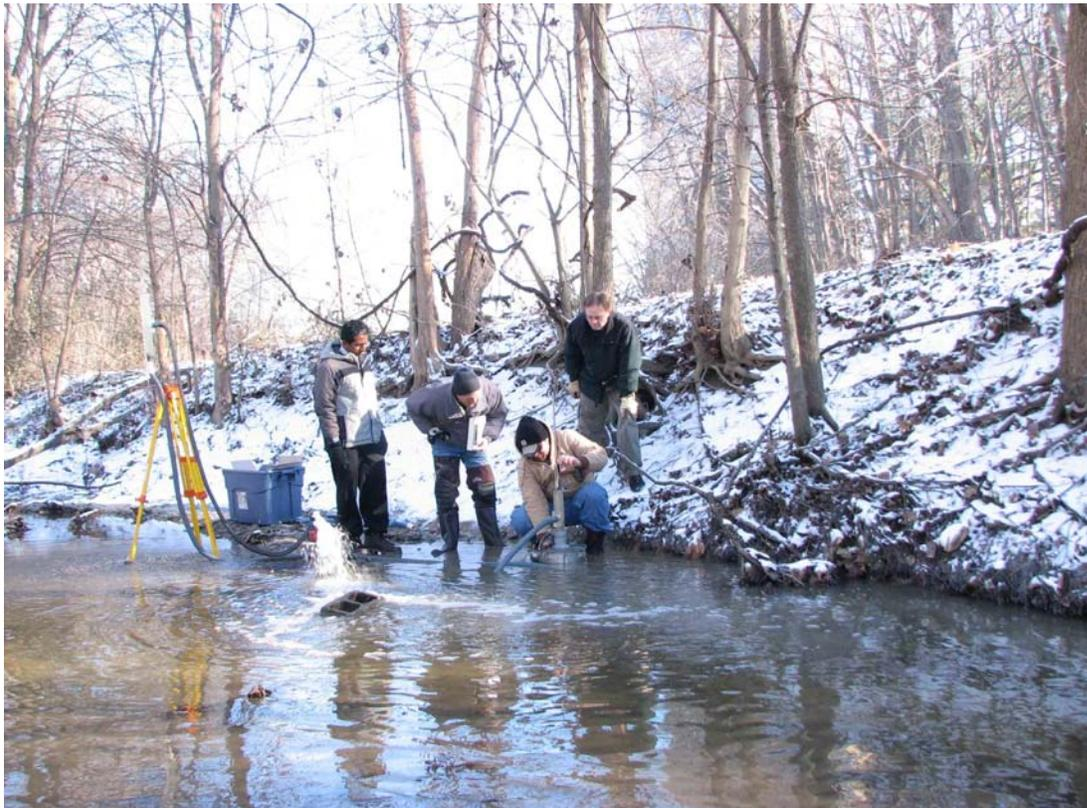
**Figure 6.2** Dr. Greg Hanson demonstrating the jet erosion test.
