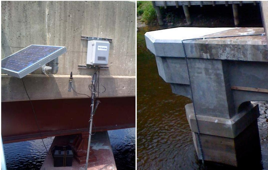
**Figures 6.11(a)** Enclosure and solar panel **(b)** Pier with conduit
