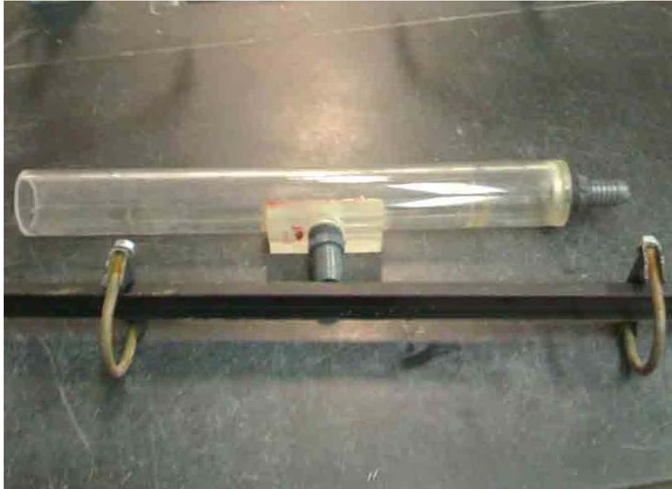
**Figure 6.5** Head pole and head tank
