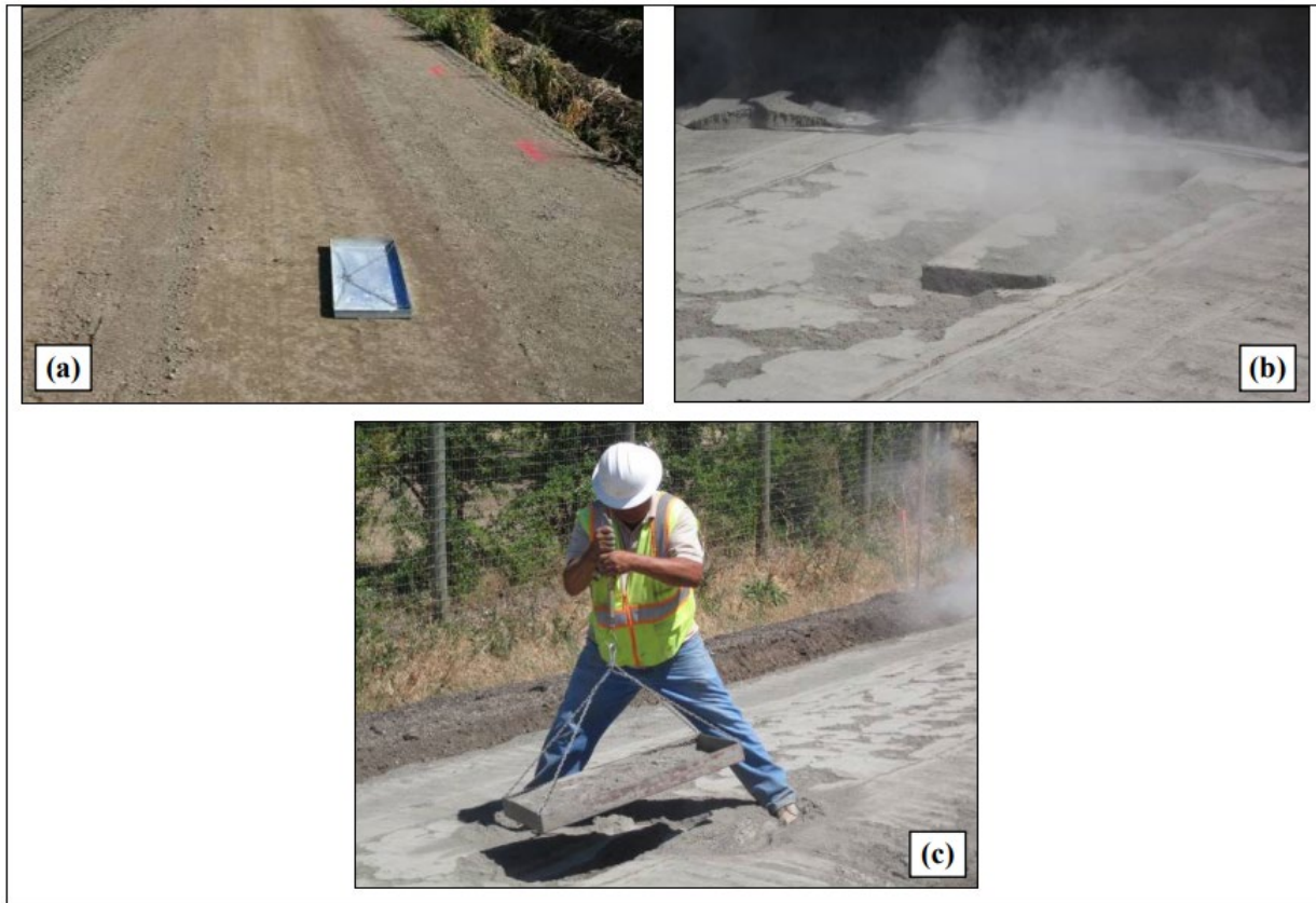
Figure 12. Checking the Chemical Substance Application Rate: (a) Place the Receptacle in the Middle of the Application Path, (b) Apply the Stabilizer, and (c) Weigh the Receptacle with Stabilizer to Determine the Application Rate (Jones et al., 2010)
