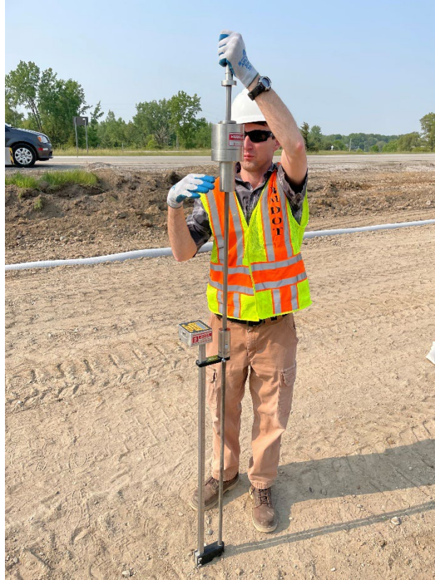
Figure 22. DCP in Operation
