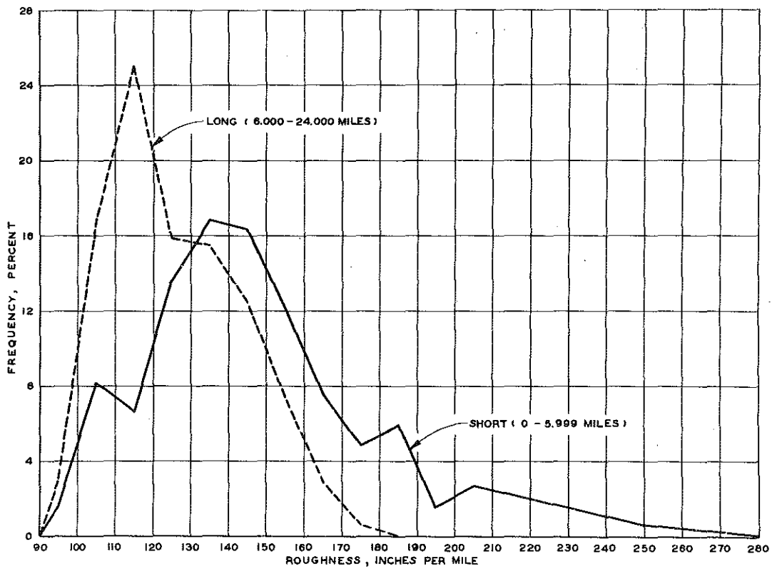
Figure 5. Frequency distributions of pavement roughness for "long" and "short" projects.
