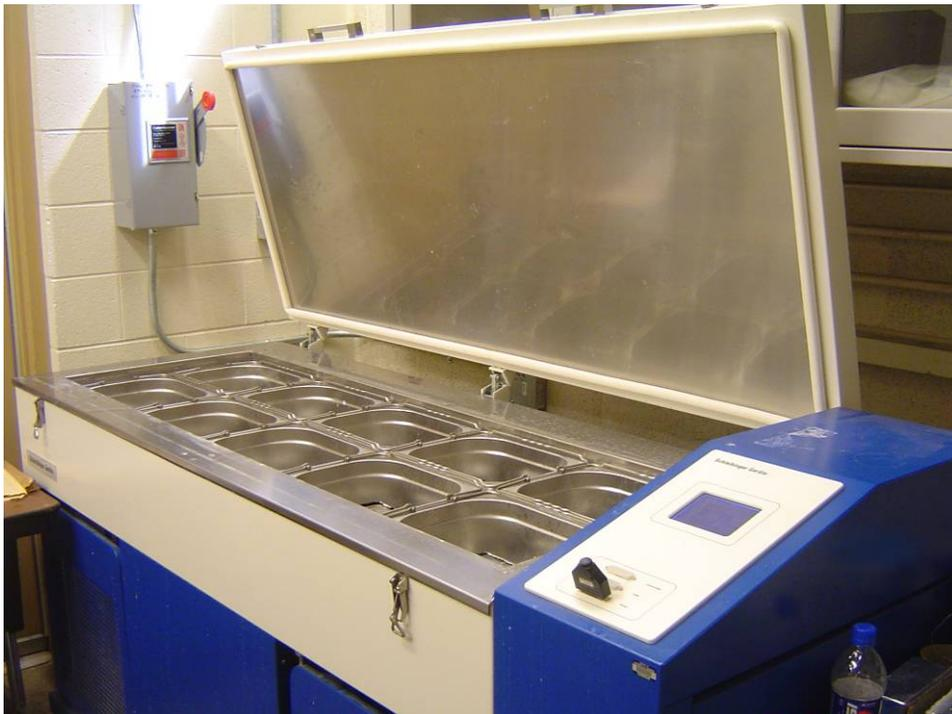
Figure 2.2 Freeze-Thaw Machine ([www.schleibinger.com](http://www.schleibinger.com))
