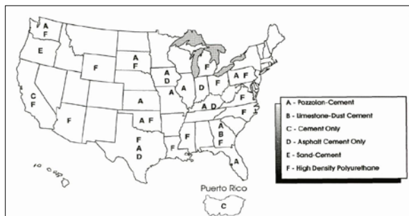
Figure 19: Typical slab stabilization materials used through the United States (American Concrete Pavement Association, 1994)
