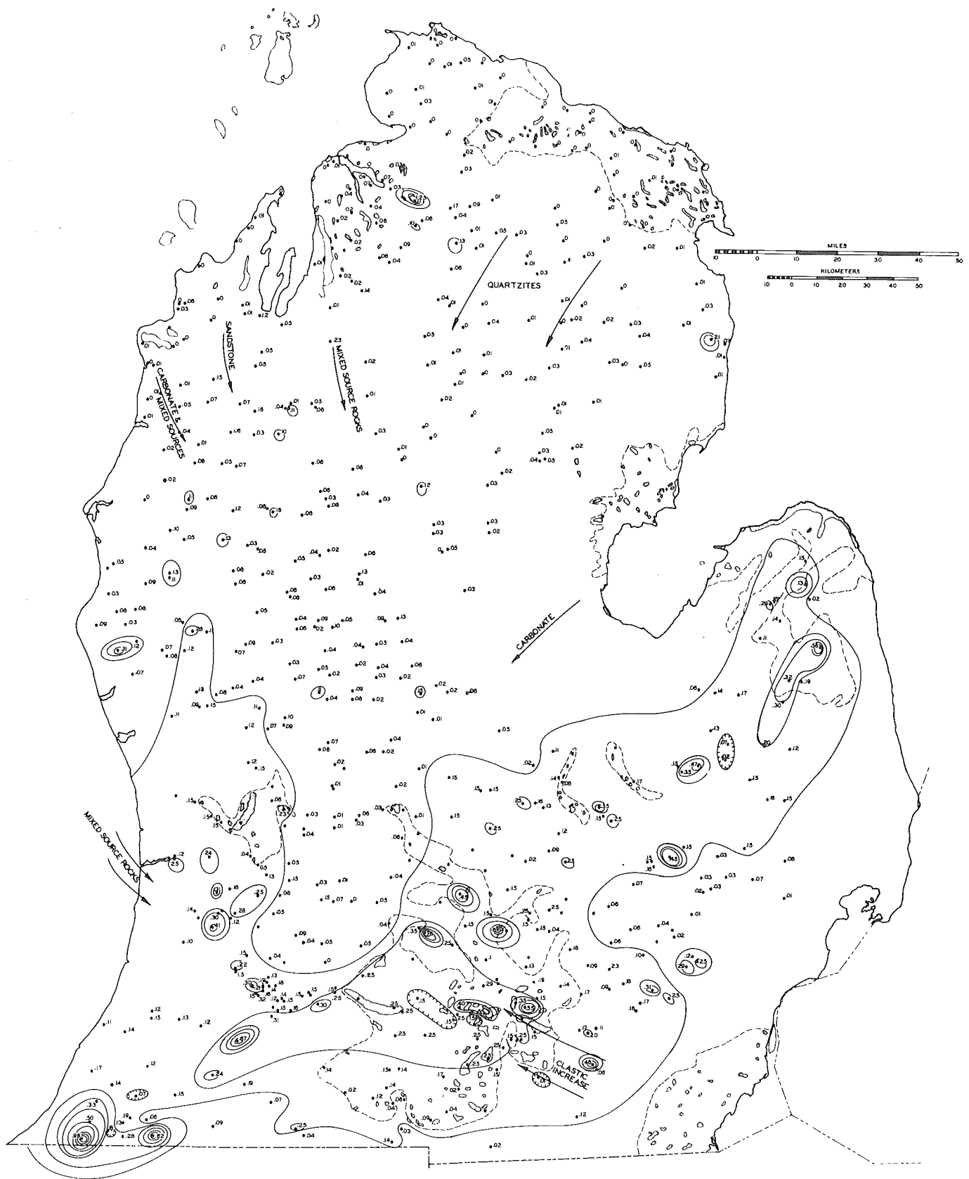
Figure 16. Ratio of clastic to carbonate rocks in glacial gravel deposits over the Southern Peninsula of Michigan (Contour interval = 0.10).
