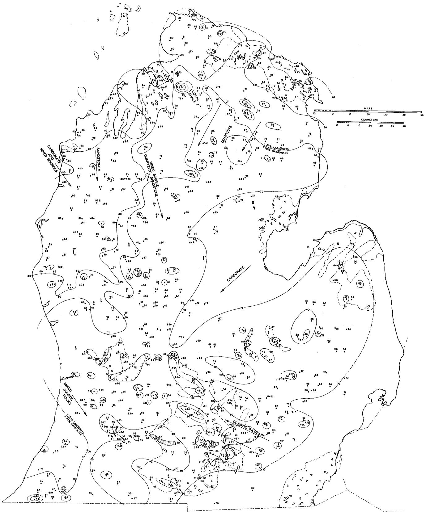
Figure 14. Distribution of non-carbonate rocks in glacial gravel deposits over the Southern Peninsula of Michigan (Values shown are percent carbonate rocks. Contours close around low values of contour interval. Contour interval = 10%).
