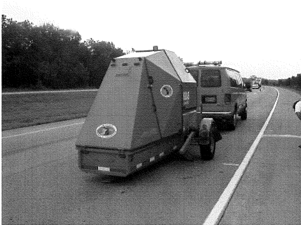
Figure 7. MDOT's FWD testing at Site 4A, US-23 SB.
