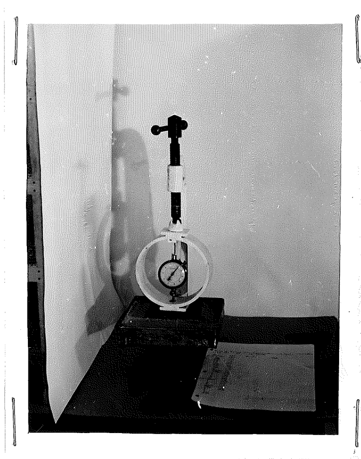
Figure 4. View of apparatus used in measuring pressures exerted by both normal and compressed wood when surrounded by water or mortar. A series of three such instruments was used in this investigation. Instrument consists essentially of a large C-clamp with suitable steel plates for sandwiching specimens, a dynamometer ring and a dial indicator registering in ten-thousandths of an inch.
