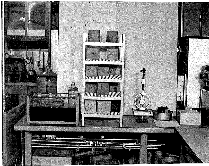
Figure 2. Center shows drying rack used for conditioning wood blocks at different stages of investigation. At left can be seen water bath for immersion of blocks. At right is one of a series of identical instruments incorporating dynamometer ring and dial indicator for measuring pressures developed in wood in contact with water or mortar.
