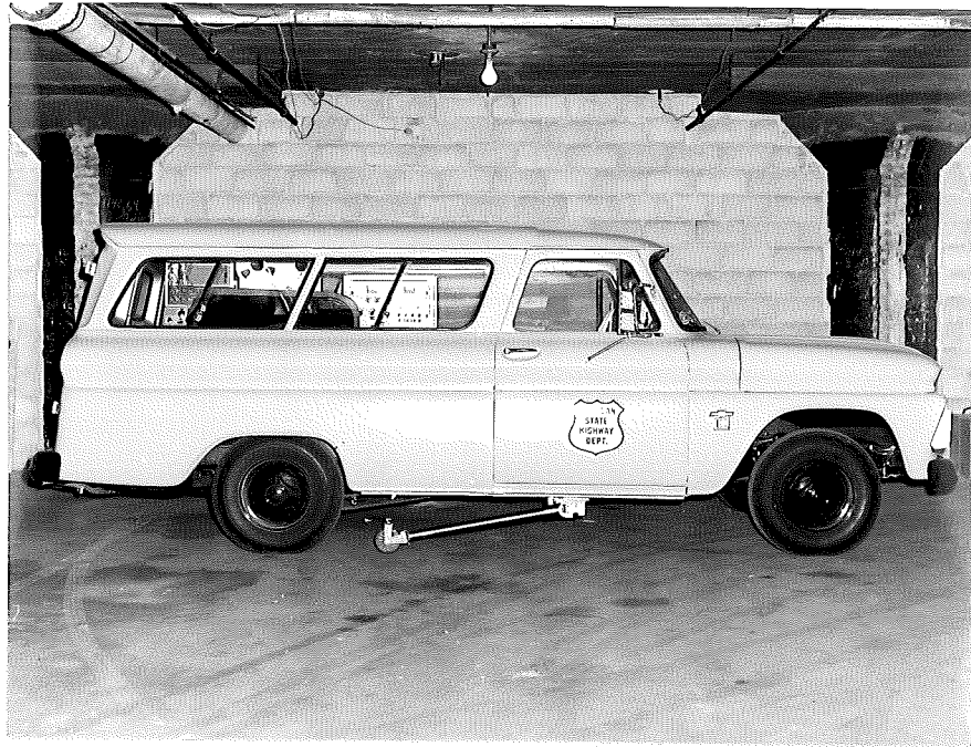
Figure 1. View of Rapid Travel Profilometer vehicle showing pavement follower arm in test position (potentiometer shaft not connected).
