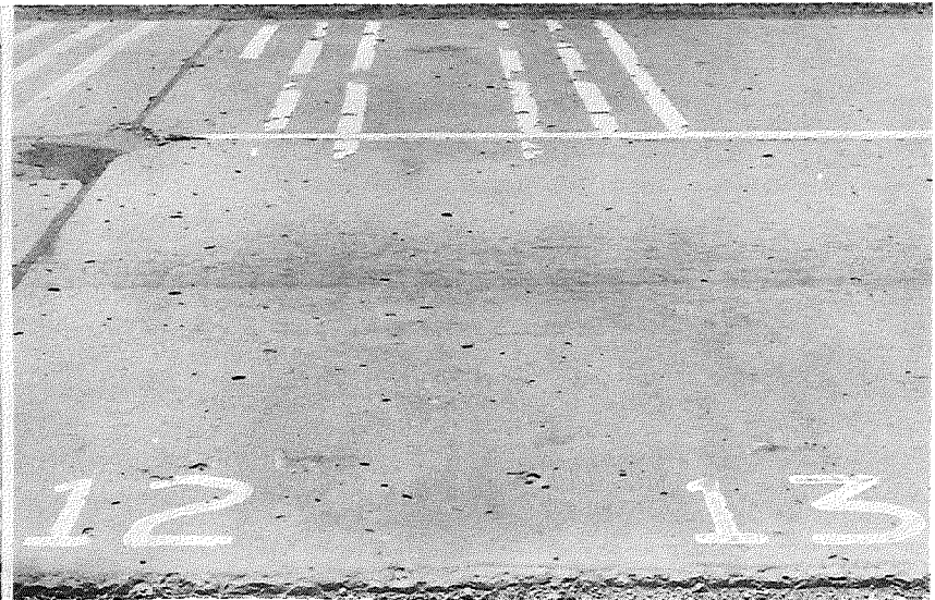
▲ February 27, 1961, after 3.4 years exposure, showing further loss of striping in passing lane.
