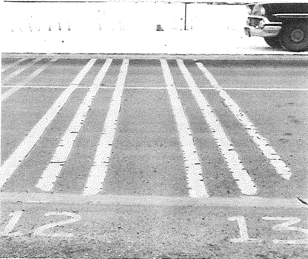
Figure 2. Progressive weathering of Catatherm thermoplastic striping being evaluated as experimental transverse stripes on black-top of US-127, south of Lansing.
