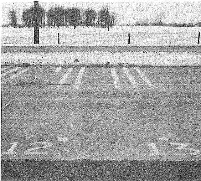
◀ Appearance of striping on January 21, 1959 after 447 days of exposure.
