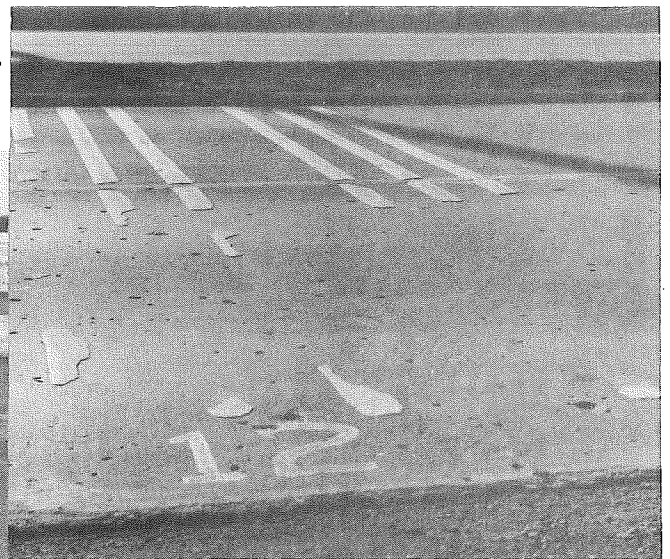
◀ Appearance of striping on January 21, 1959 after 447 days of exposure.
