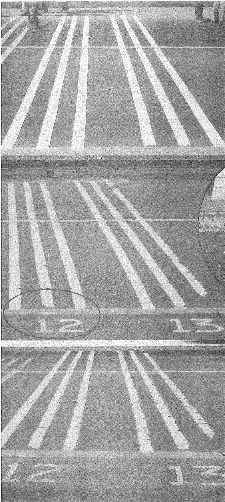
Figure 3. Catatherm Thermoplastic experimental striping on black top of US-127, Lansing - Holt Test Area.
