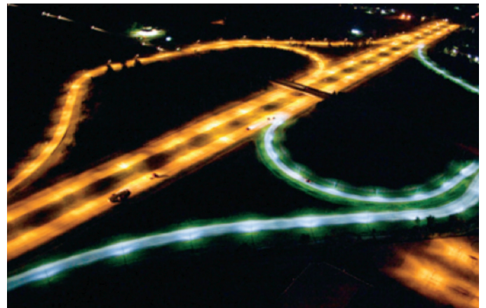
Differences in the color temperatures of traditional high-pressure sodium lamps (yellow/top) and LEDs (blue/bottom) stand out on an I-275 interchange west of Detroit.
