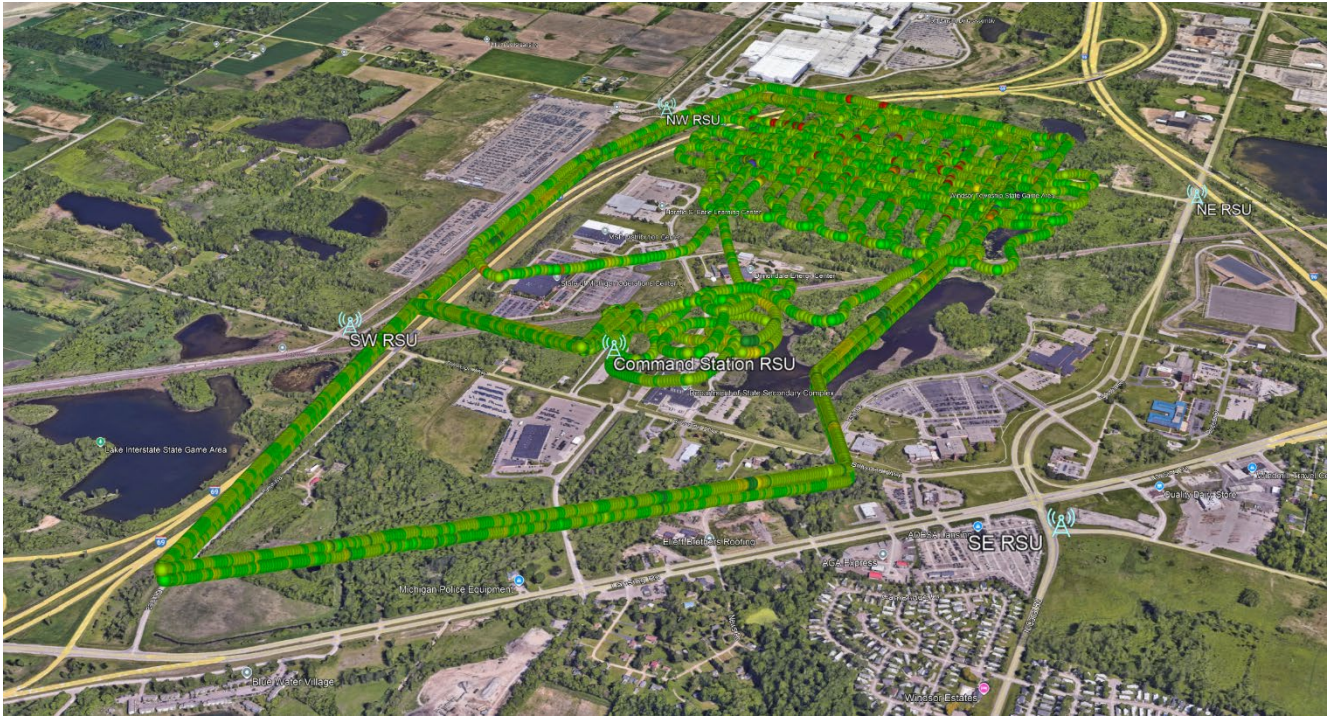
FIGURE 15. OVERHEAD VIEW OF COMMUNICATIONS RECEIVED BY ONE OR MORE RSU; COLOR CODED BY TIME DELTA SINCE LAST RECEPTION
