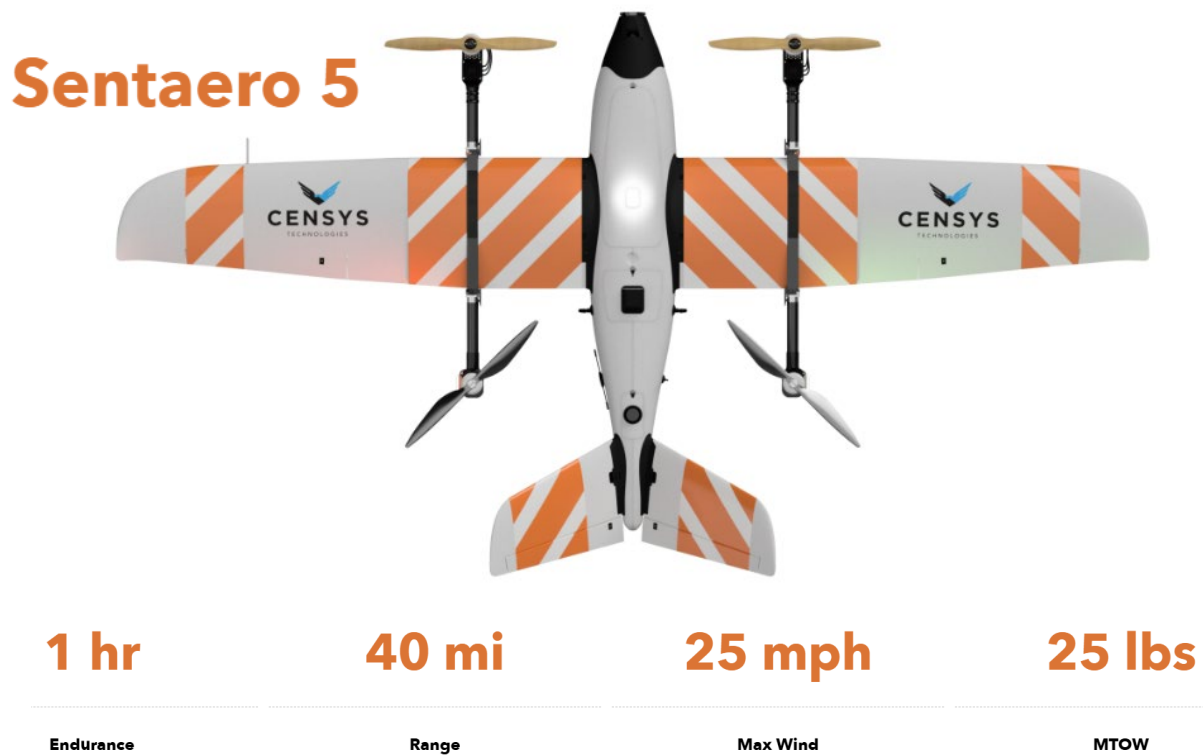
FIGURE 10. CENSYS SENTAERO 5 UAS PLATFORM USED IN THE DEMONSTRATION
