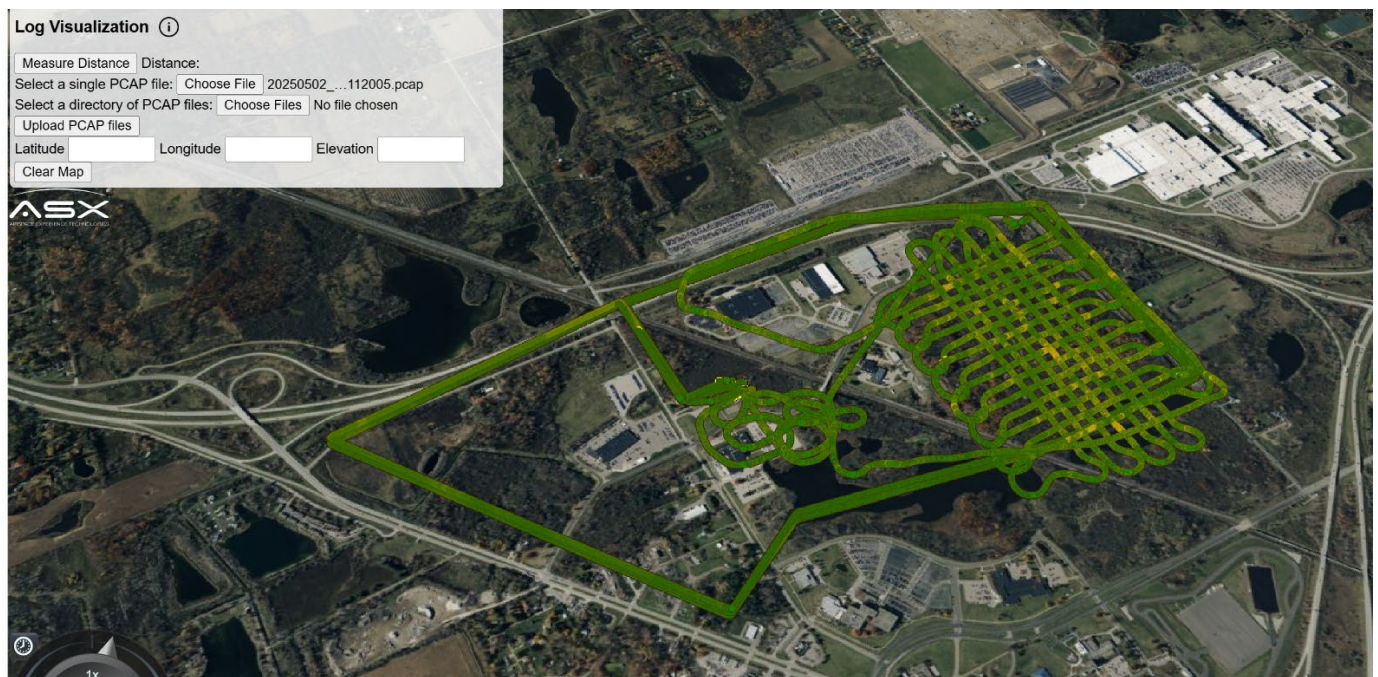
FIGURE 13. EXAMPLE TRANSMISSION LOCATION YELLOW DOTS OVERLAYED WITH GREEN RECEPTION DOTS
