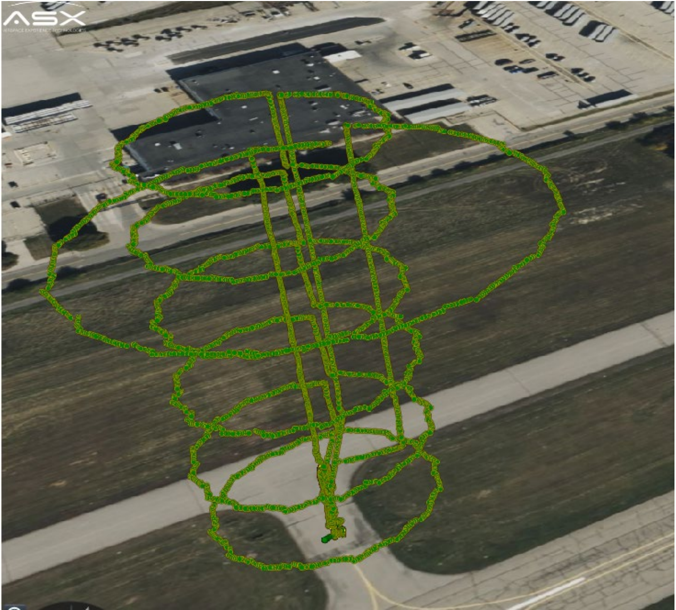
FIGURE 20. RECEPTION FROM THE WEST RSU SHOWS GREEN DOTS COVERING YELLOW DOTS FOR THE ENTIRE FLIGHT
