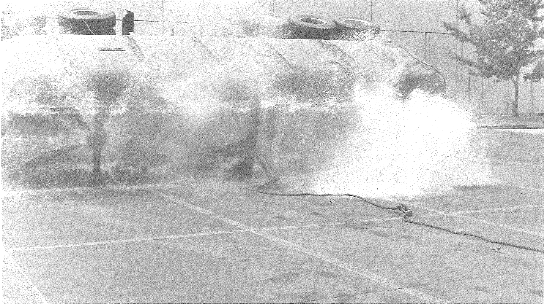
Figure 5.35. Moment of impact in the 4th experiment with clamp-ring-type manhole cover dislodging at far right. Note that the vehicle is reversed in this view, right/left, from the transducer layout diagram in Figure 5.34.
