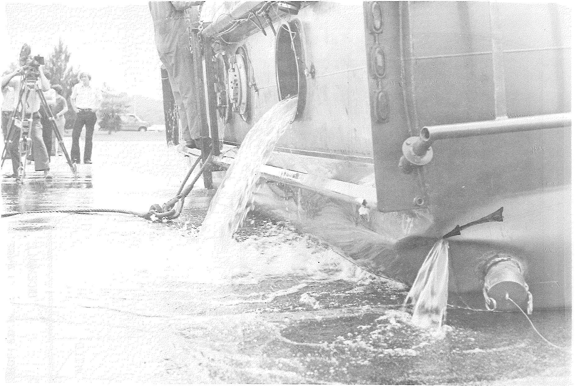
Figure 5.7. Weld seam split (arrow) observed following rollover experiment discussed in Section 5.2.
