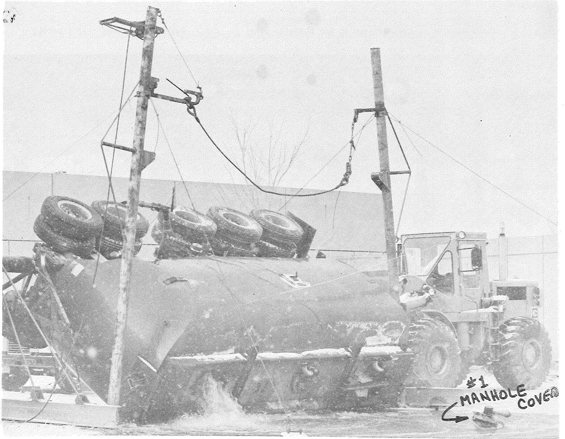
Figure 5.20. Severe rollover test, time = impact + 1 sec.
