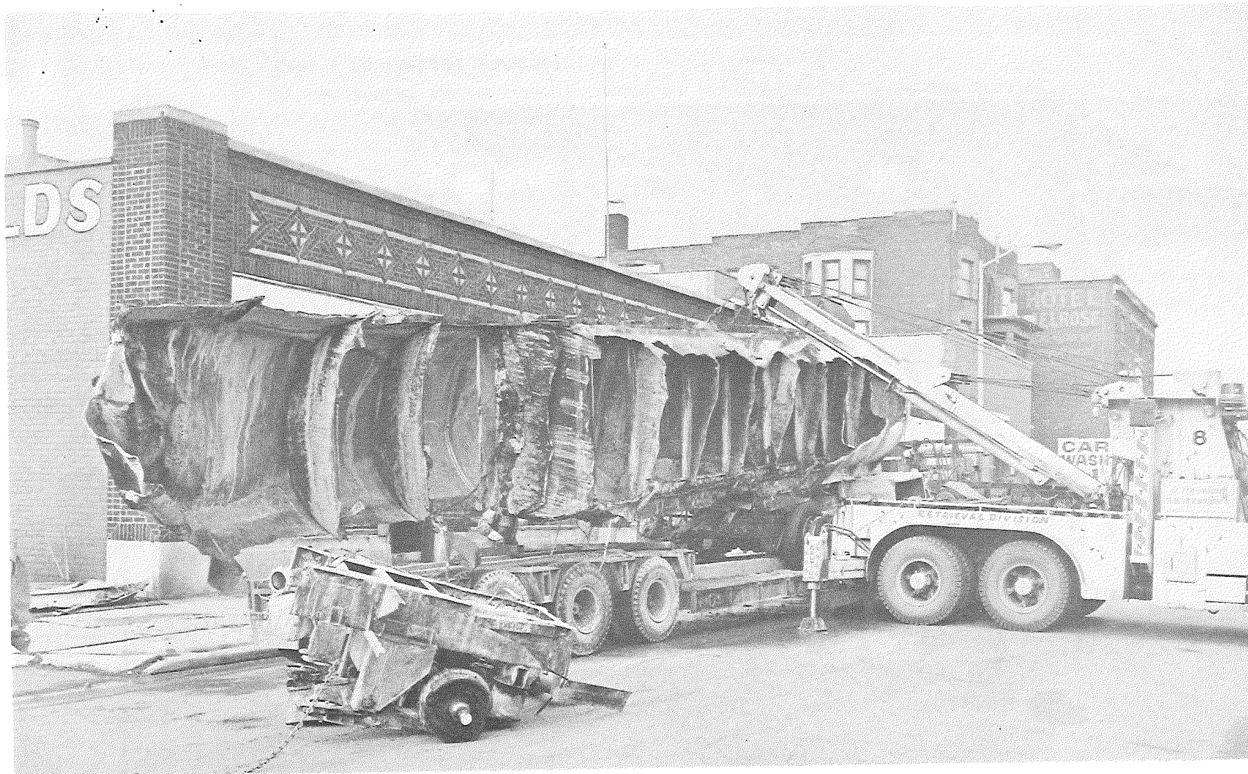
Figure 5.12. Remains of aluminum-shell gasoline tanker following rollover and fire (courtesy of S-K Services).
