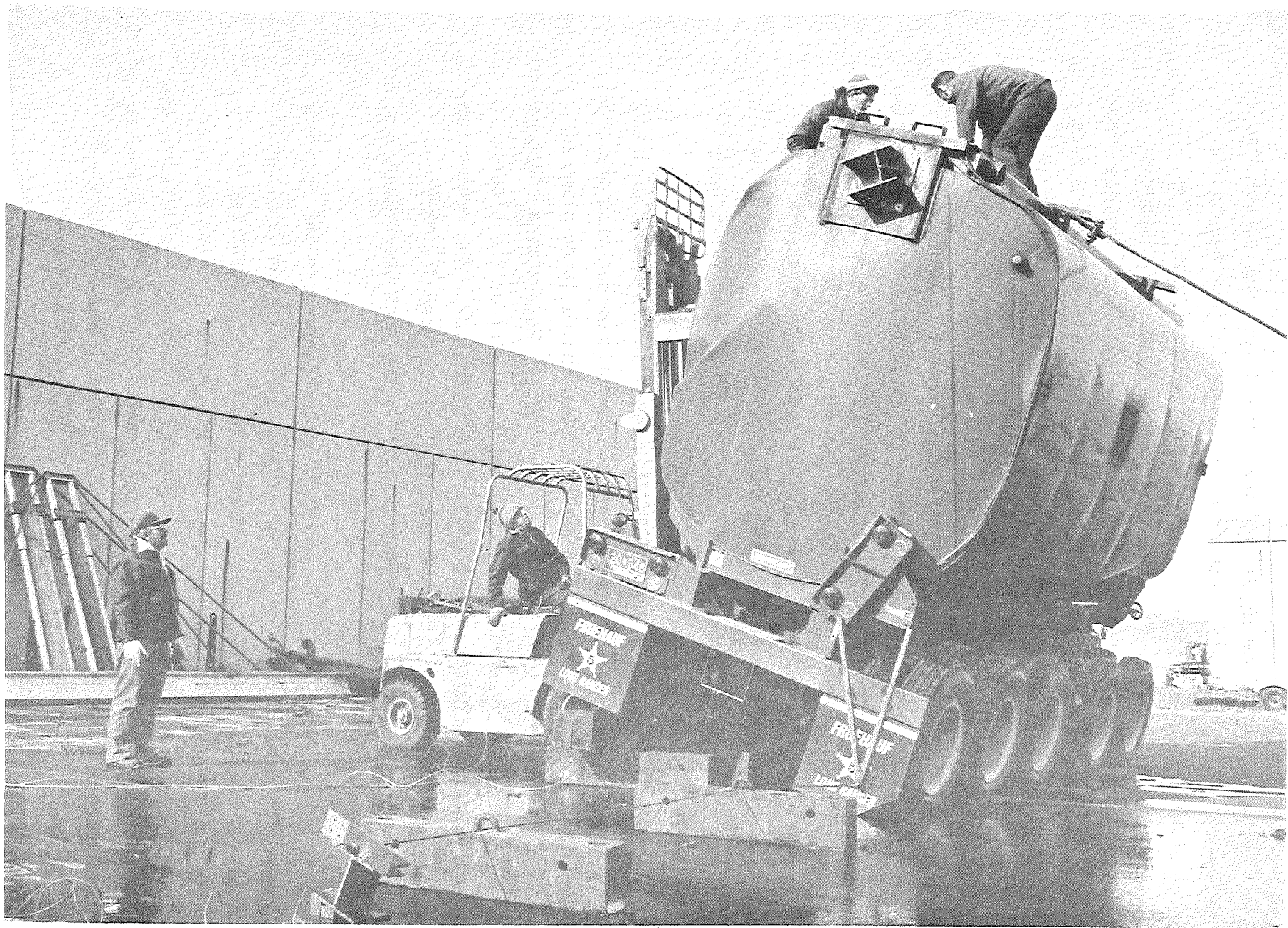
Figure 5.25. Tanker inclined to an initial roll angle of 15 degrees for "tipover" experiment.
