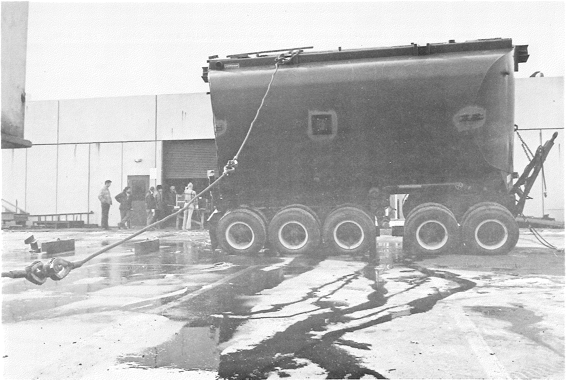
Figure 5.26. Tanker with tow cable used to initiate tipover.
