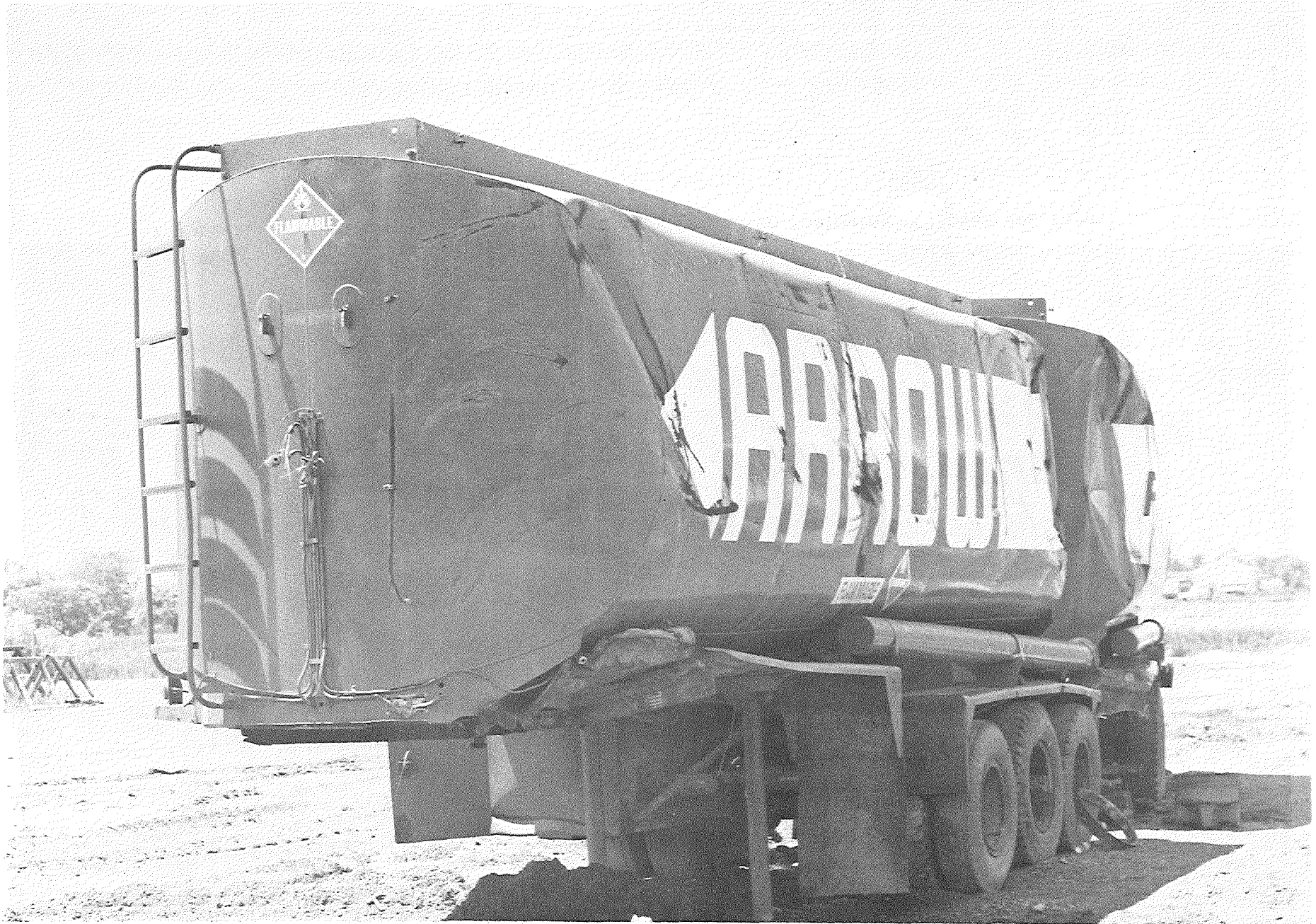
Figure 5.11. Double tanker showing deeply indented leading corner of second trailer's tank - no leakage occurred.
