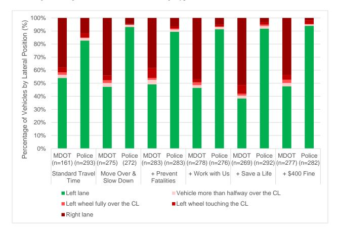
Figure 27. Percentage of Downstream Passenger Vehicle Lateral Position by Type of Service Vehicle
