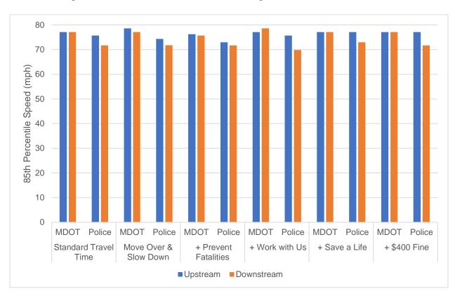
MOSD message with an additional message of WORK WITH US had the highest drop in speed between the upstream and downstream of DMSs, 5.9 mph.
