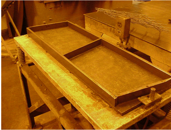
Wear track slab forms
