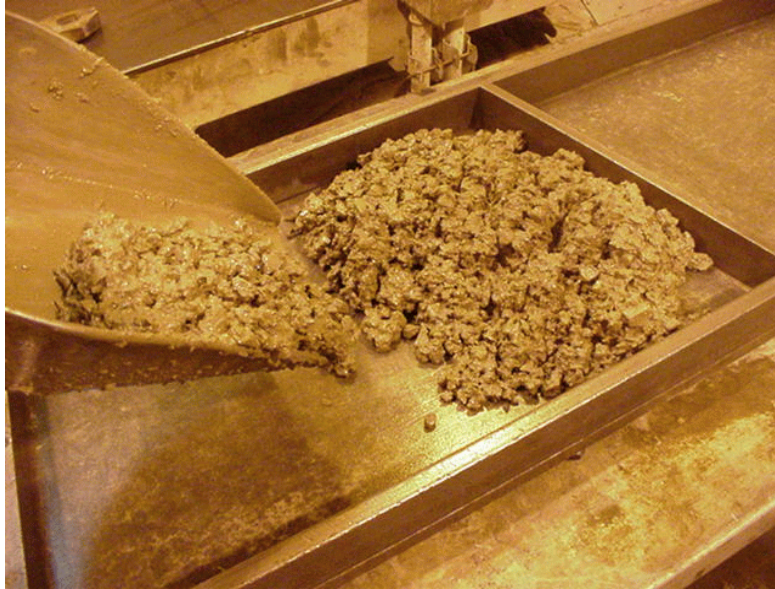
26A concrete mixture being placed in form
