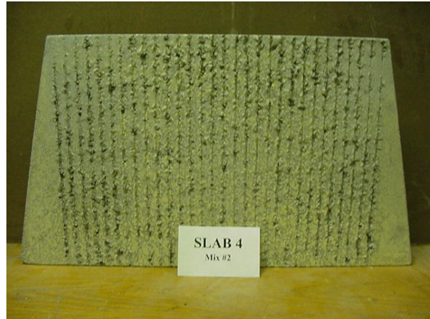
Slab 4 tined finish (left), and slab 4 with curing compound (right)
