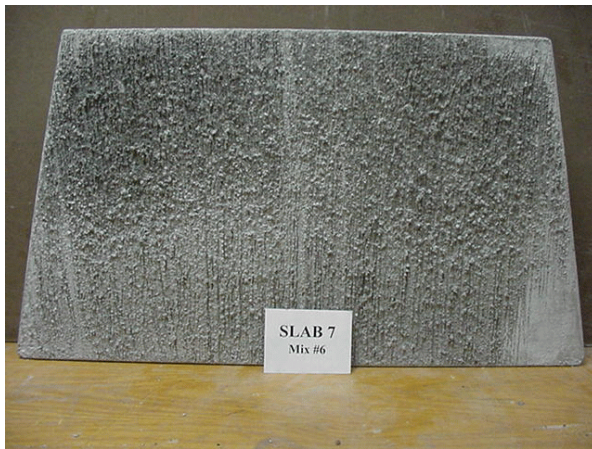
Slab 7 with transverse astroturf drag texture (left), and coated with white curing compound (right)
