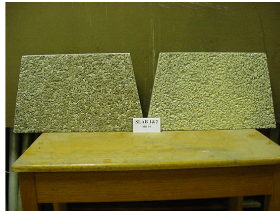
Slab 2 (right) is coated with curing compound
