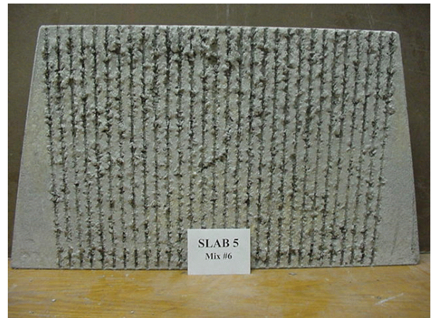
Slab 5 coated with curing compound
