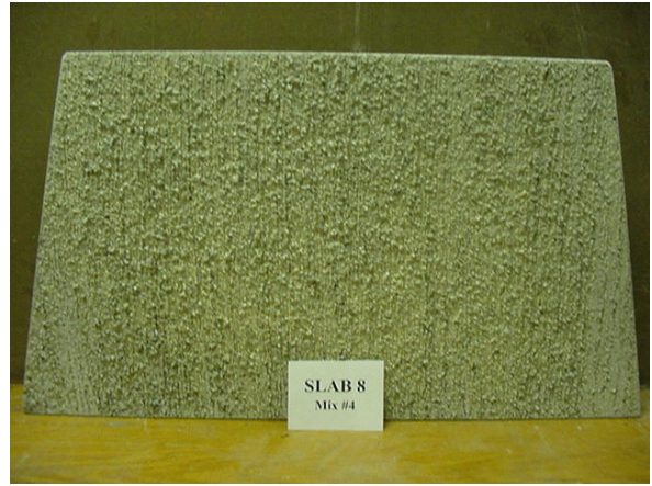
Slab 8 (left) with astroturf drag texture and coated with curing compound (right)
