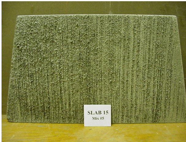
At left is slab 15 with an astroturf drag surface texture, and, at right, is slab 15 coated with curing compound
