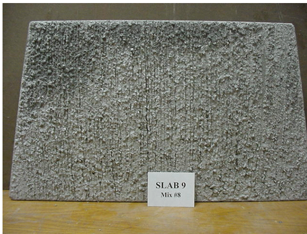
Astroturf drag texture on slab 9
