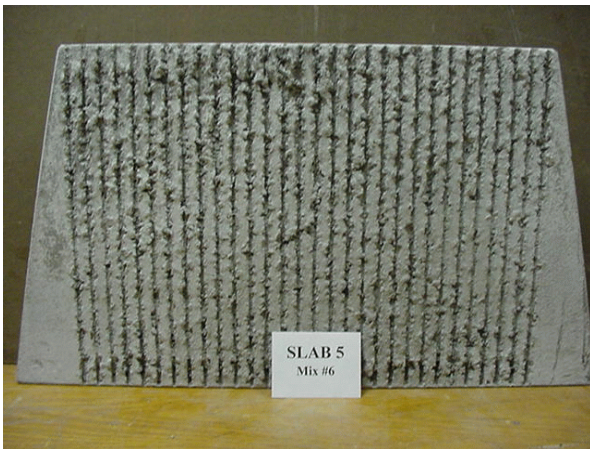
Tined surface texture on slab 5
