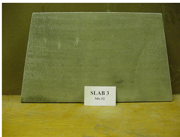
Photo at left shows slab 3 smooth trowel finish, at right is slab 3 with curing compound applied
