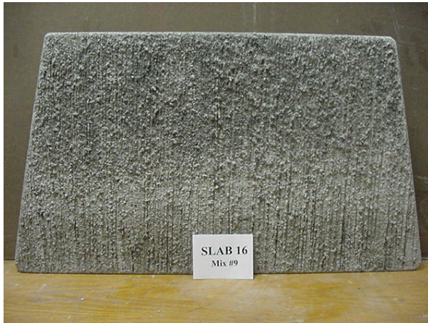
Astroturf drag finish on slab 16 (left), and slab 16 coated with curing compound (right)
