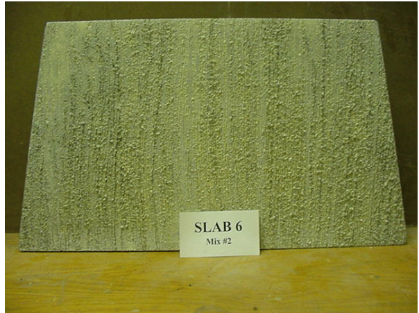
Slab 6 with astroturf drag finish (left) and coated with curing compound (right)
