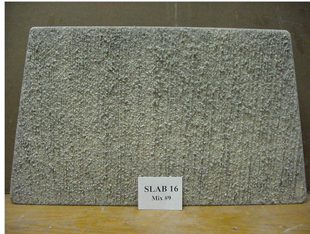
Astroturf drag finish on slab 16 (left), and slab 16 coated with curing compound (right)
