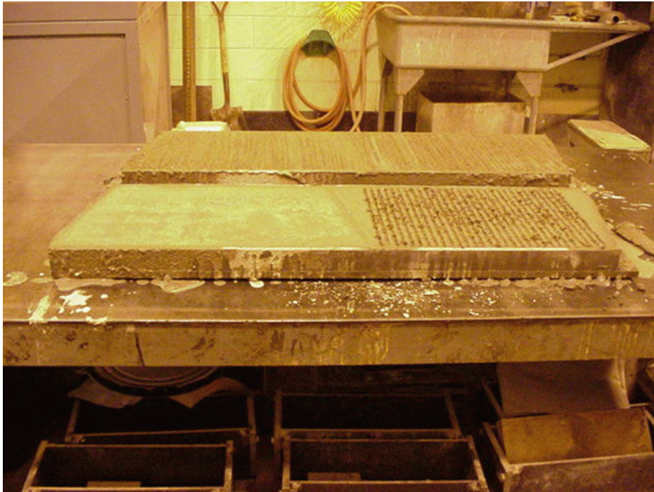
Smooth trowel finish ( bottom left ), transversely tined finish ( bottom right ), astroturf drag finish ( top )
