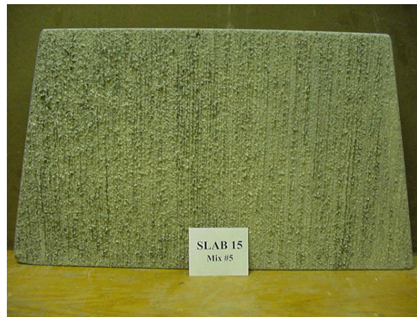
At left is slab 15 with an astroturf drag surface texture, and, at right, is slab 15 coated with curing compound
