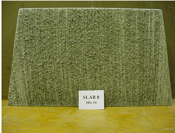
Slab 8 (left) with astroturf drag texture and coated with curing compound (right)
