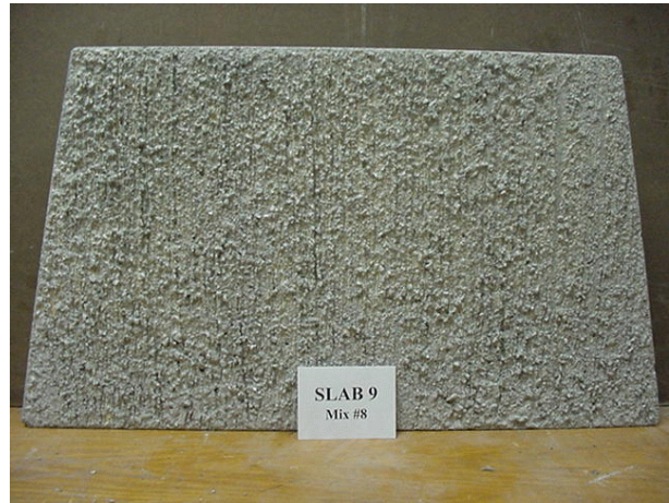
Slab 9 coated with curing compound
