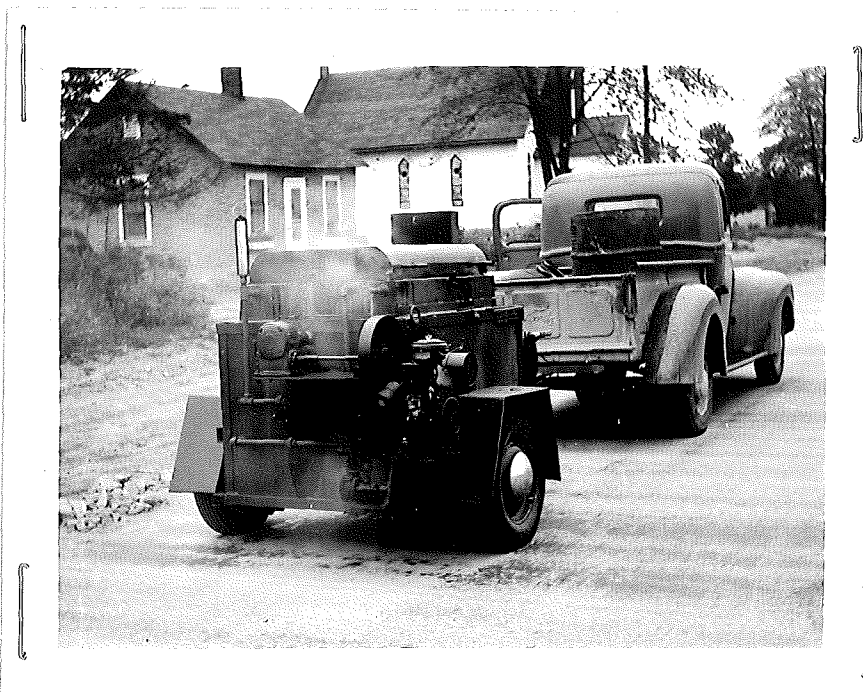
Illustration No. 2 Note smoke haze as a result of overheating the oil bath
