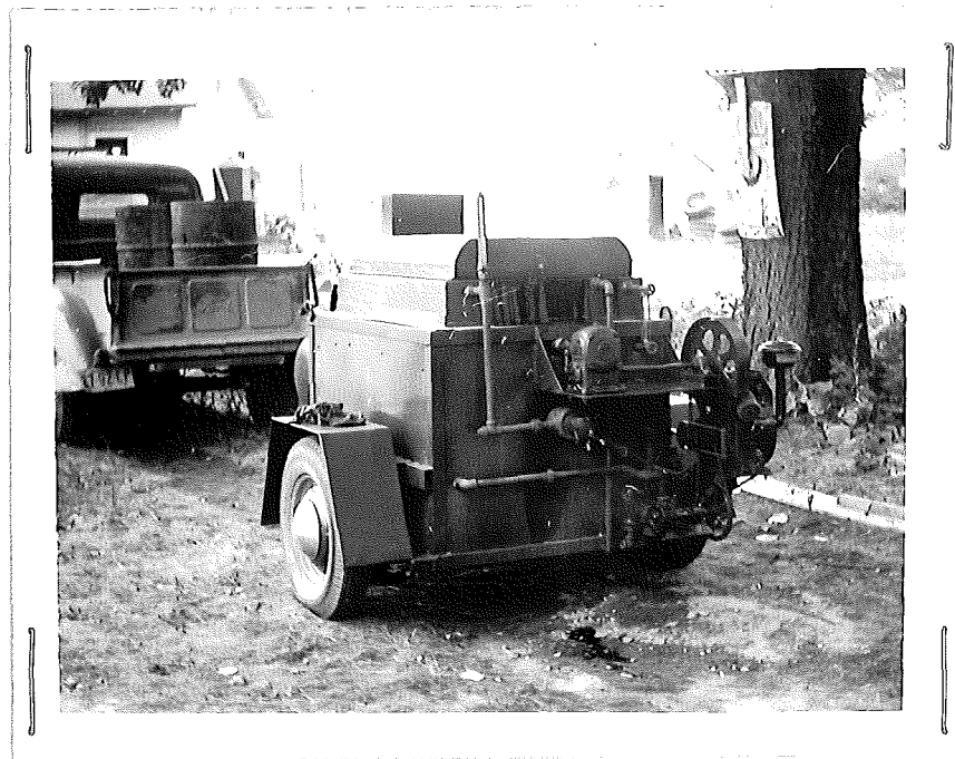
Illustration No. 1 Rubber Compound Kettle, Model B-115, designed and built by W. G. Chausse, Manufacturer, of Detroit, Michigan
