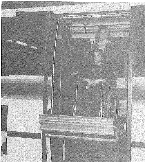
Rear Door Steps in Lift Position
