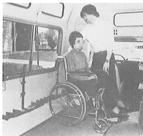
Figure 36. Wheel-locking Wheelchair Securement Devices.
