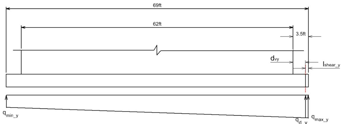
Distance from end of the footing to the critical section for shear
