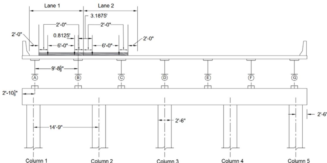
(a) Lane and Load Positions to Develop the Maximum Positive Moment in the Pier Cap
