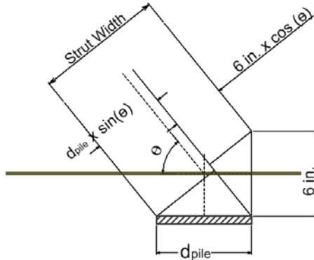
Node 1 is a CCT node at which a tie intersects only from one direction. The surface at which the diagonal strut meets the node is called the strut-to-node interface.
