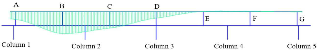
Influence line to develop the maximum girder reactions to obtain the maximum shear in the pier cap (the maximum shear developed at Column 2)
