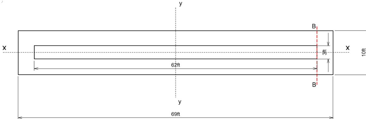
Section modulus of the footing about y-axis
