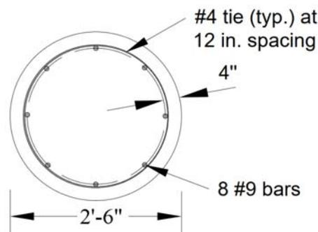
Note: Tie lap is not shown in the figure for clarity.
