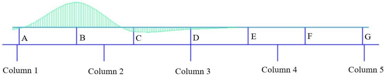
Influence line to develop the maximum girder reactions to obtain the maximum negative moment in the pier cap (the maximum negative moment developed at Column 2)
