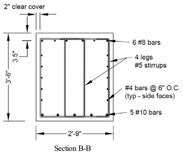
Note: Certain details are not shown in this drawing for clarity of the main reinforcement. Refer to the MDOT Bridge Design Guides for additional details.
