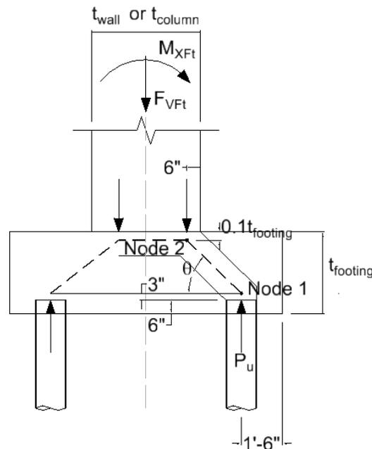
The centroid of the top chord is assumed to be located at a distance of  $1/10^{\text{th}}$  the footing thickness below the top of the footing. There are several options that the designer may consider when placing the top chord. Please refer to **FHWA-NHI-17-071** *Strut-and-Tie Model (STM) for Concrete Structures* for additional details. Also, Step 7.6 of this series of examples provides more details on this topic.
