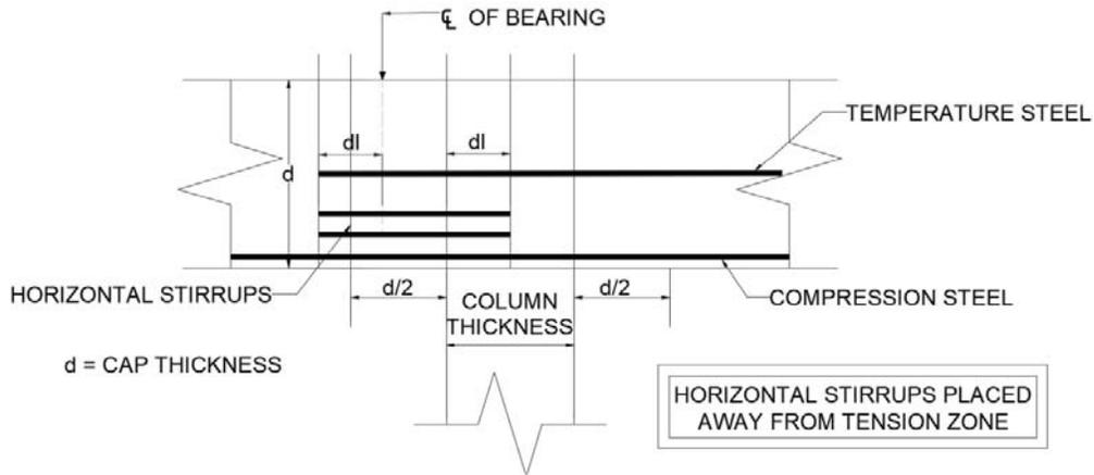
In this example, none of the bearing points are located within a distance of  $d/2$  from the face of the pier columns. However, for illustrative purposes, it is assumed that a bearing point lies within a distance of  $d/2$  from the column face.
