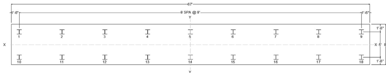
Section modulus of the pile group about x-axis
