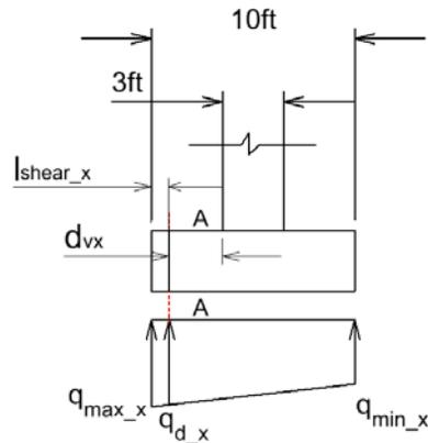
Distance from end of the footing to the critical section for shear
