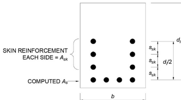
Distance from the extreme compression fiber to the centroid of the extreme tension steel
