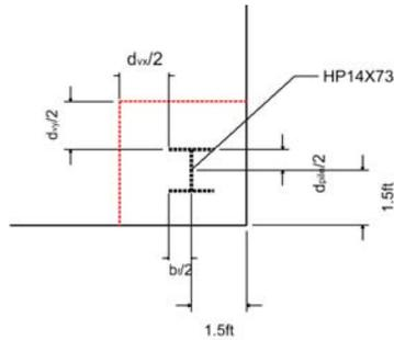
Ratio of long-to-short sides of the pile cross-section
