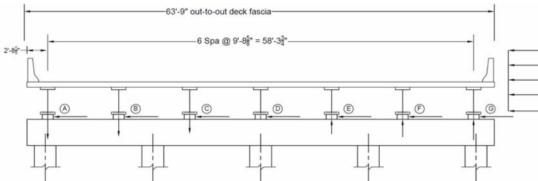
The following calculations show the moments about the longitudinal axis of the bridge due to the transverse wind loads on the superstructure:
