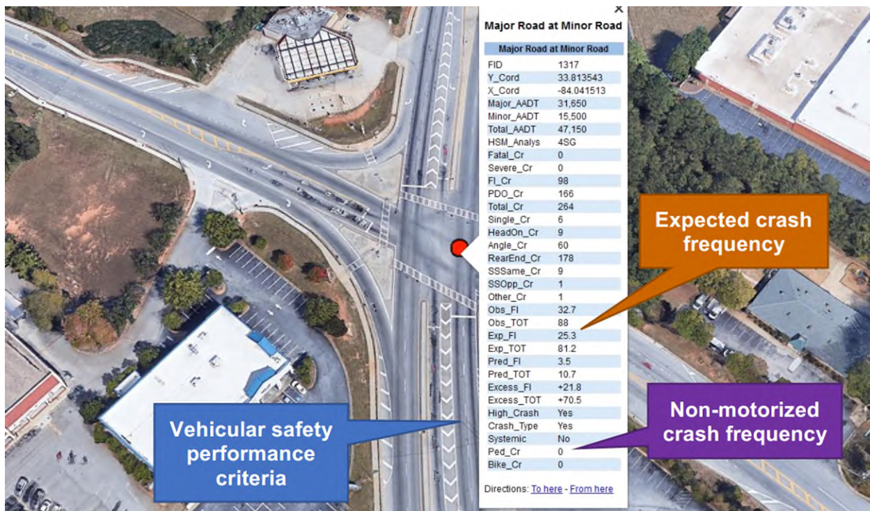
Figure 13. Four-Legged Signalized Intersection Selected for Traffic Signal Modernization
