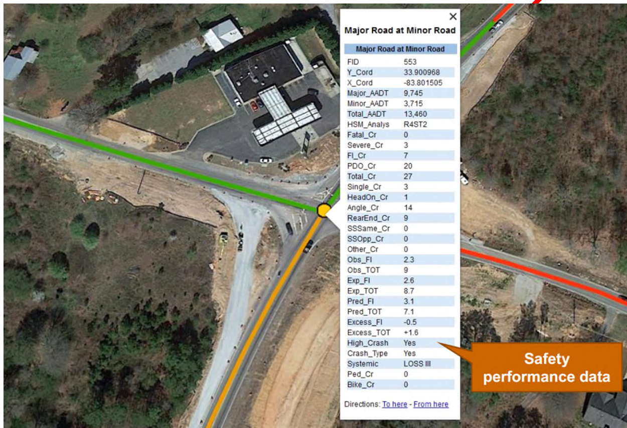
Figure 18. Four-Legged Unsignalized Intersection Identified for Traffic Control Modification
