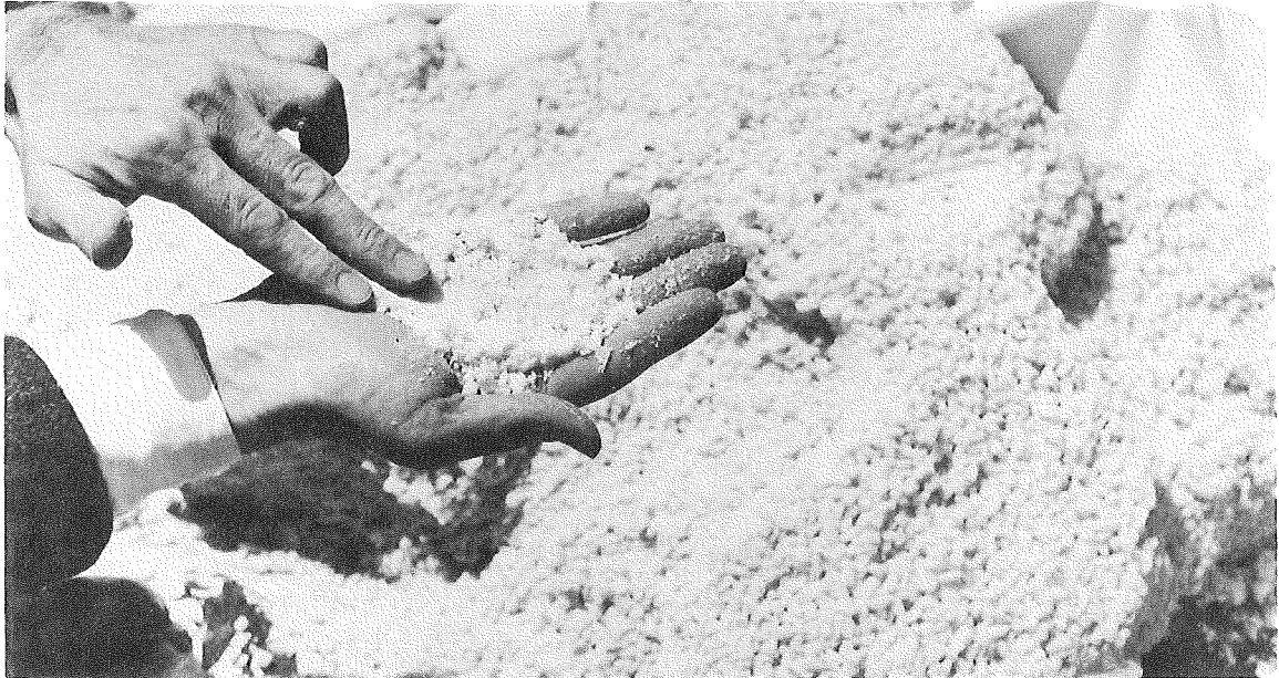
Figure 7. Breakup of Cubidow to precompacted condition (covered First Sample after 9 months of exposure).
