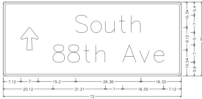
D1-2 (1.2) 40 mph or more; 1.63" Radius, 0.75" Border, White on Green; Arrow A-7 - 9.13" 90°; [South] D; [88th Ave] D;
