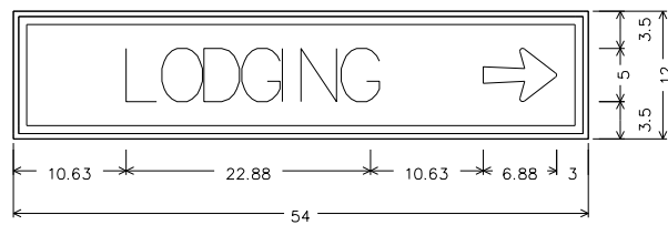
E11-15b; 0.75" Inner border White, 1.50" Radius, 0.50" Outer border, Blue on Blue; [LODGING] White C; Arrow A-5 - 6.88" 0° White;
