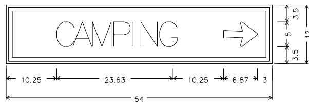
E11-15d; 0.75" Inner border White, 1.50" Radius, 0.50" Outer border, Blue on Blue; [CAMPING] White C; Arrow A-5 - 6.88" 0° White;
